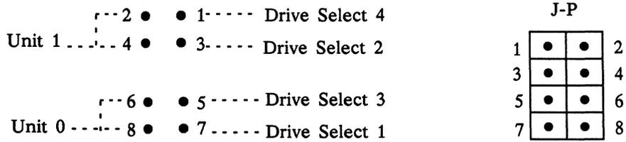
Figure 8-9. Jumper Block J-B
