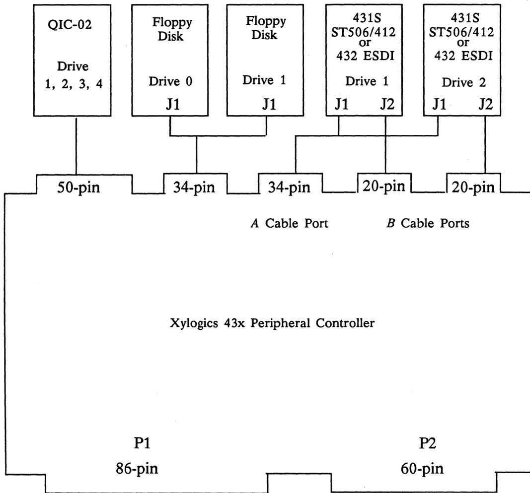
Figure 8-14. Multiple Drive Connection Diagram
