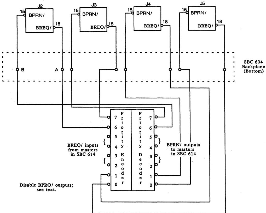
Figure 8-13. Parallel DMA Priority
