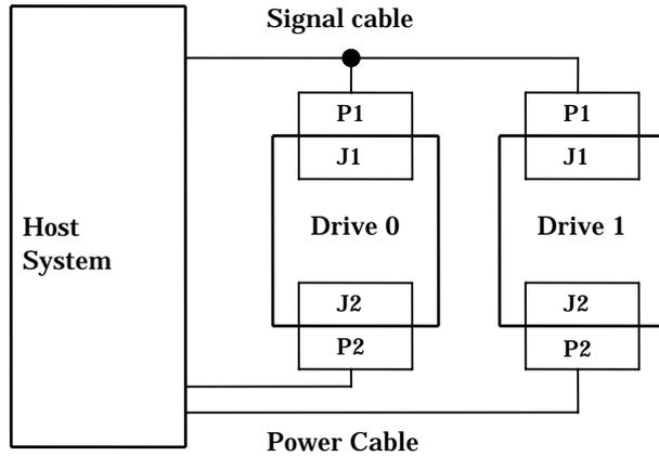
Fig.4.1 Cable Connections
