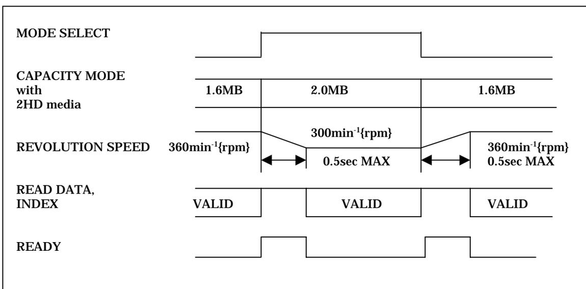
Fig.3.3 Capacity Mode Switching
