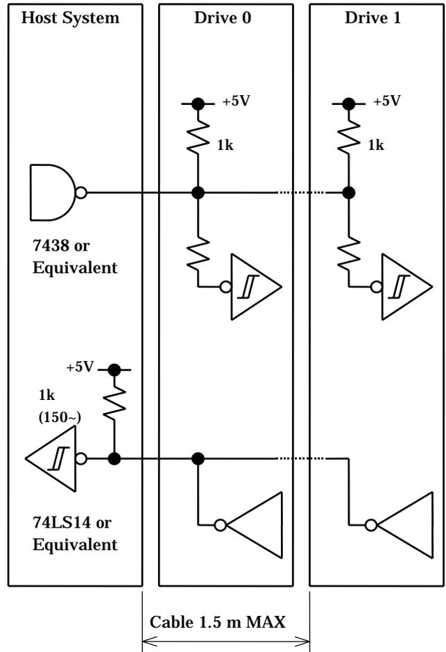
Fig. 3.7 Interface Circuit
