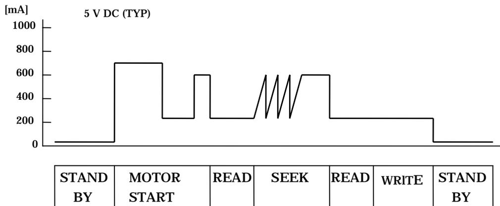
Fig.3.13 Current Waveform
