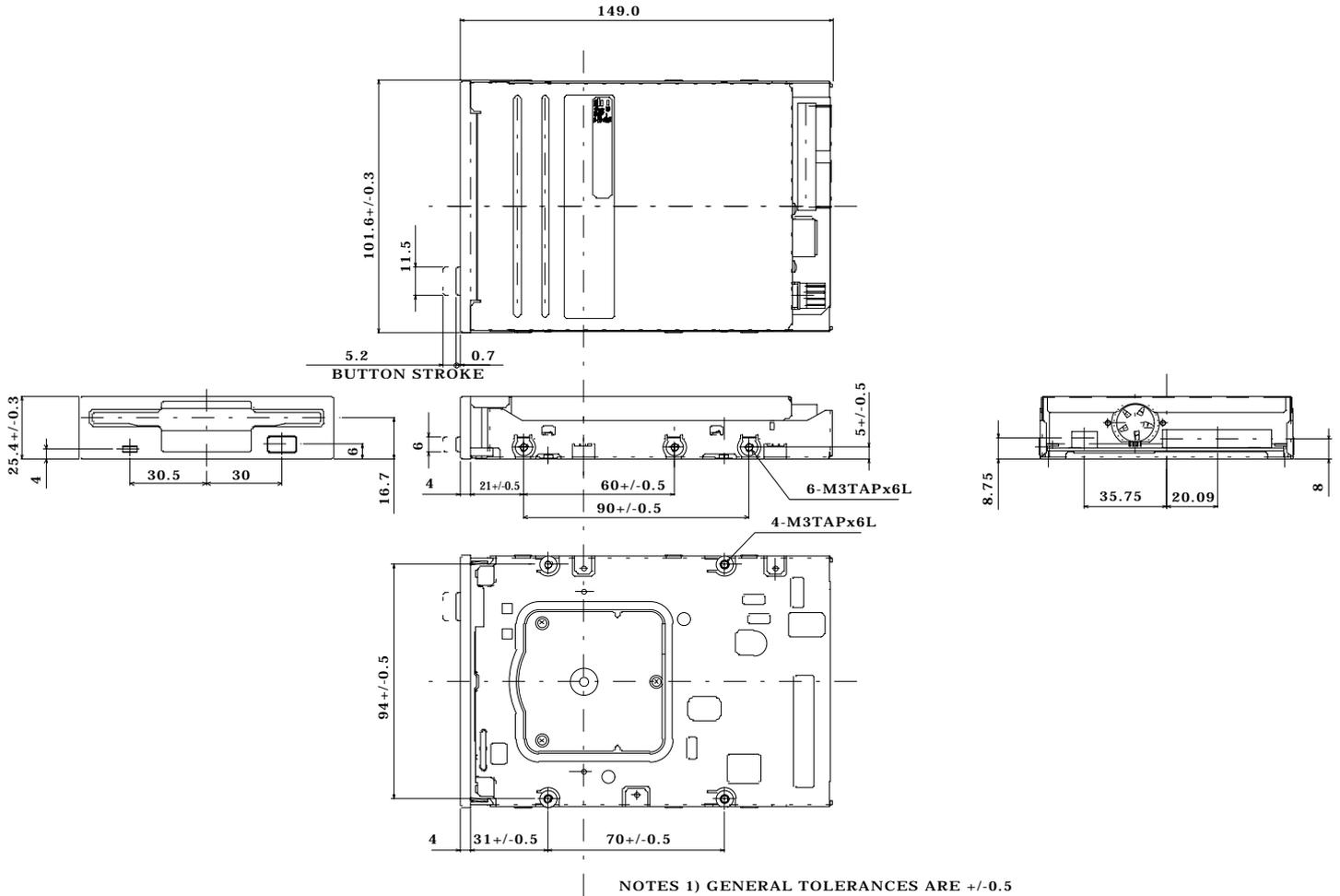
**Fig. 5.1 Mechanical Dimensions**
