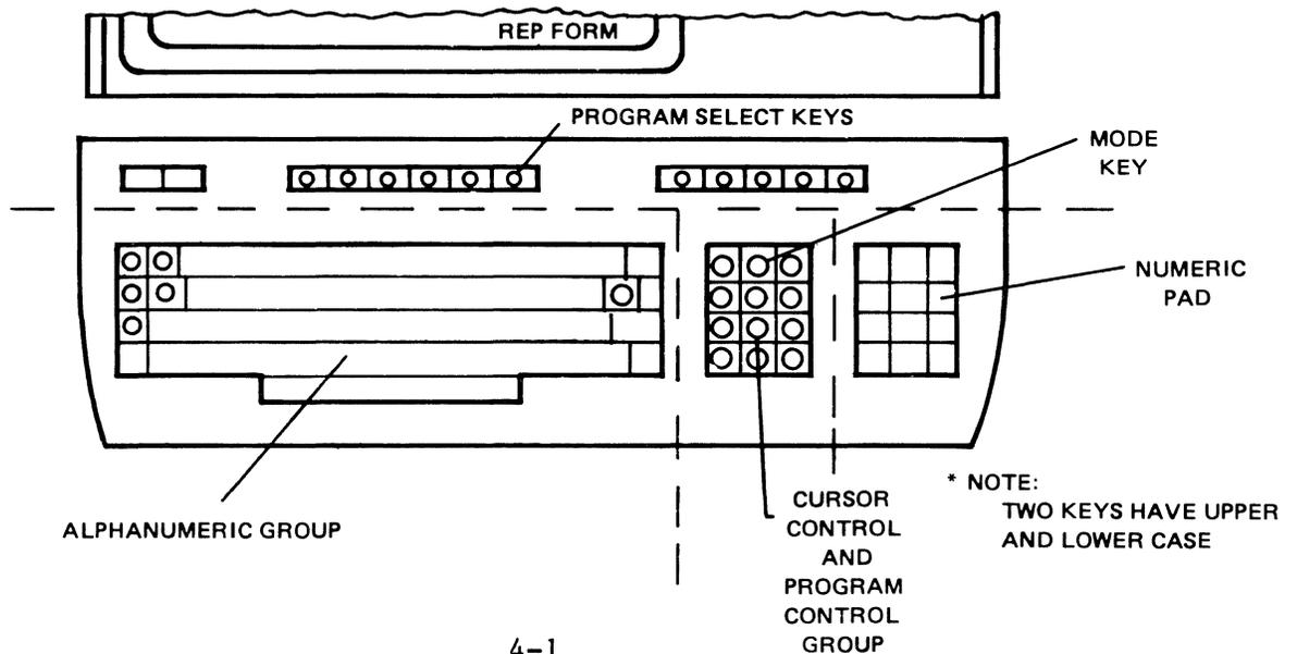
MODE Key - the MODE key is the most important key on your ZENTEC 9003. It provides the way to change the terminal from one program mode to another, and therefore, the means by which the programmability feature of the terminal is used. Depressing the MODE key causes the CONTROL MODE to be selected.
