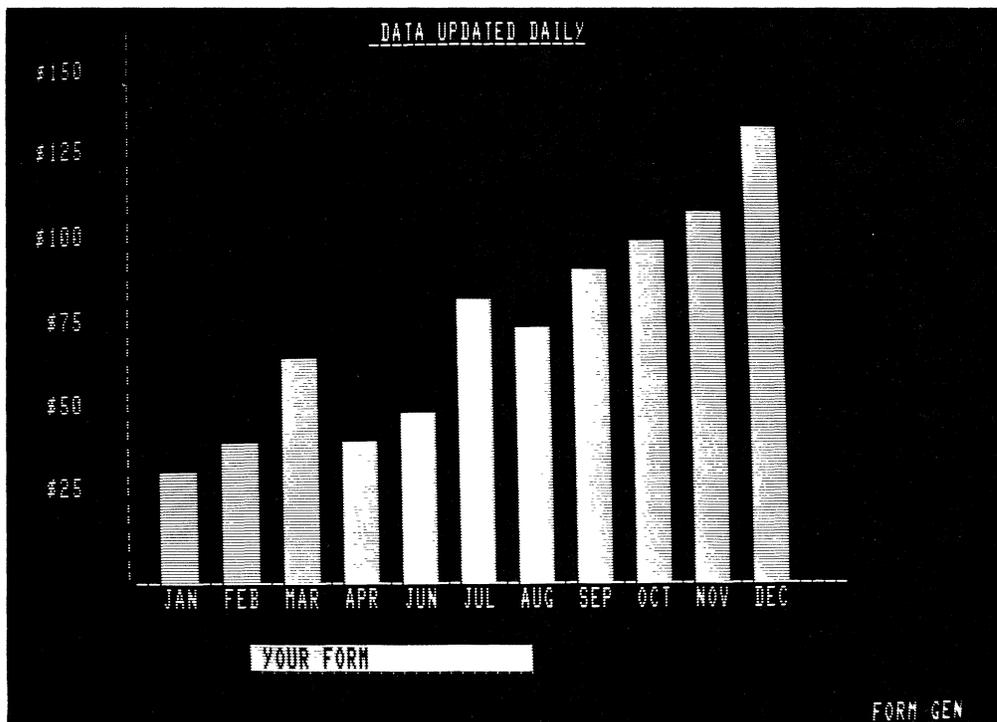
Figure 1-2. 9003 Display showing use of enhance charateristics for form generation and/or graphics.
