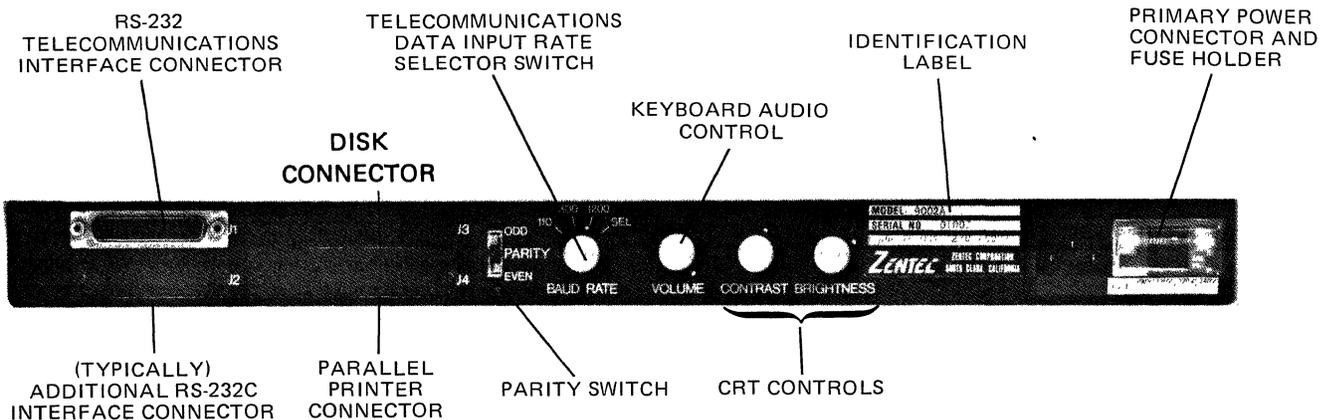
FIGURE 2-1 Rear Control Panel.
