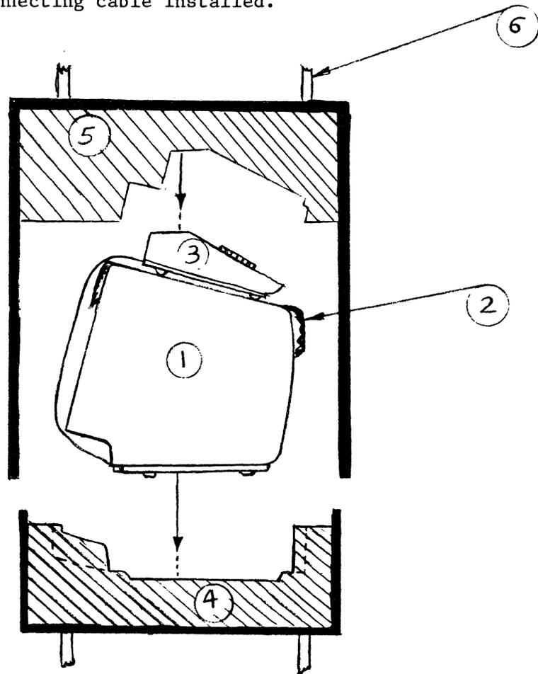
**W A R N I N G:** Be careful when unpacking the terminal not to overstress the keyboard cable and do not disconnect the keyboard cable.
