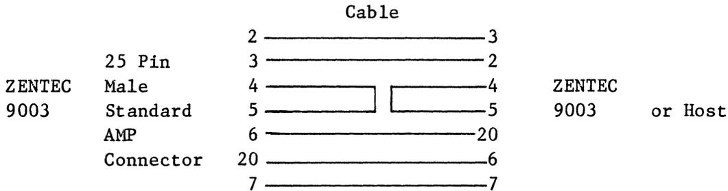
External Cable RS-232C Pin Interconnections when operating ZENTEC 9003's With a Modem.
