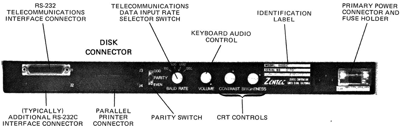
FIGURE 3-1 Rear Control Panel.
