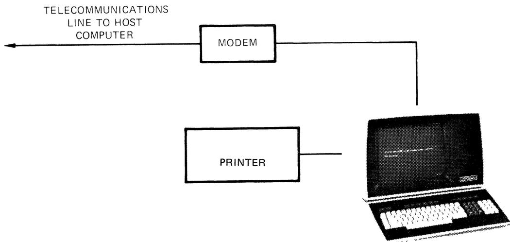
Figure 1-5. Typical 9003 System telecommunications installation.
