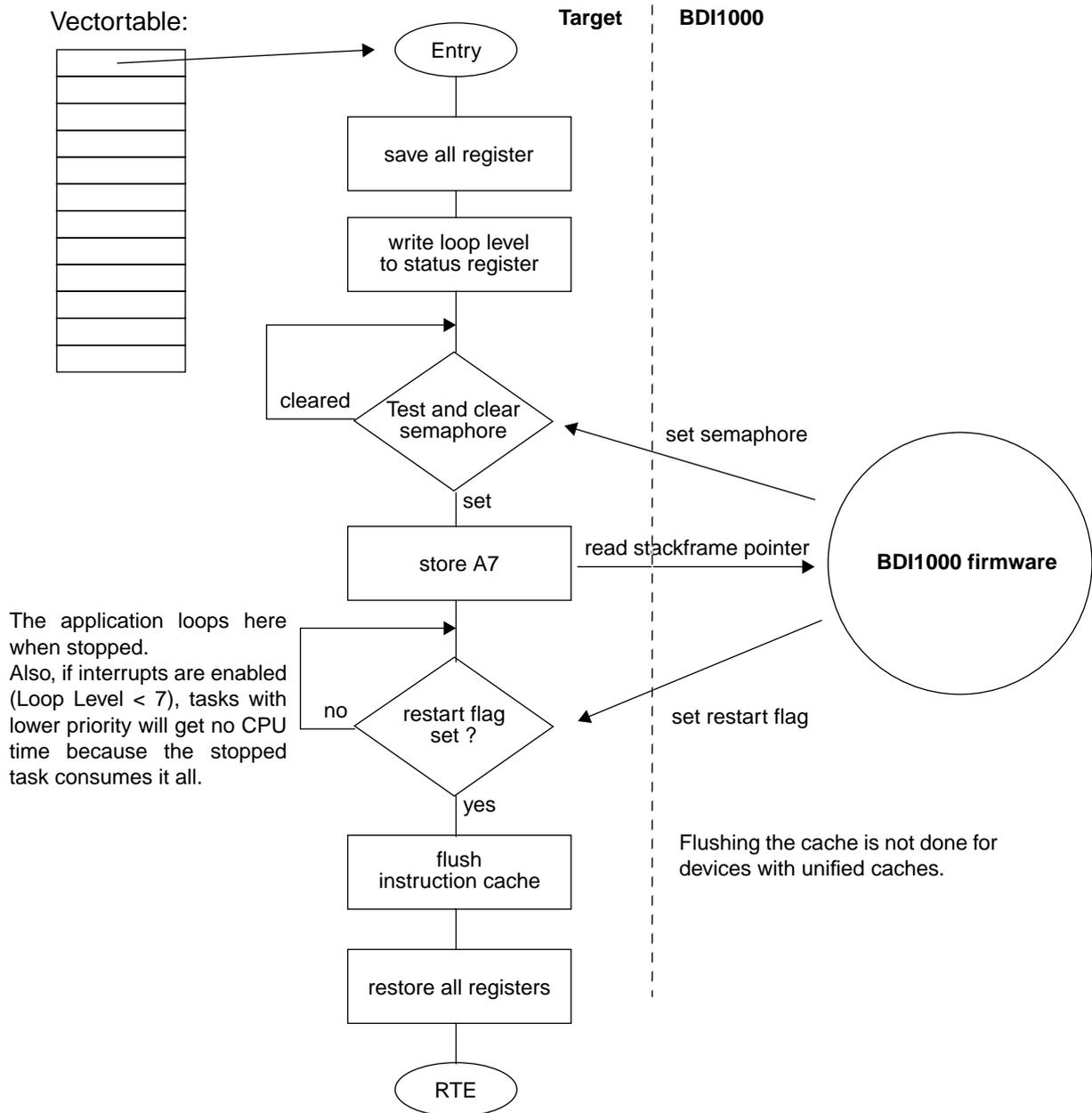
The ColdFire is never frozen because it is possible to access target memory via the BDM interface while the CPU is running.
