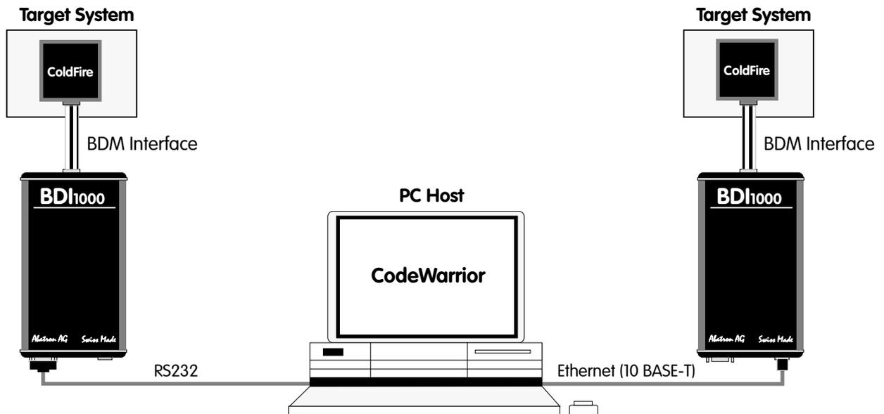
The BDI1000 adds Background Debug Mode features to the CodeWarrior debugger environment from Metrowerks. With the BDI1000, you control and monitor the microcontroller solely through the stable on-chip debugging services. You won't waste time and target resources with a software ROM monitor, and you eliminate the cabling problems typical of ICE's. This combination runs even when the target system crashes and allows developers to continue investigating the cause of the crash.
