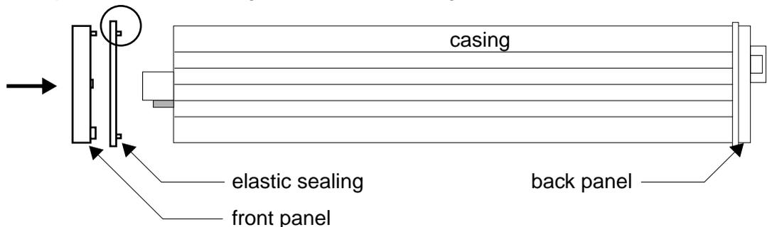
5.3 Mount the screws (do not overtighten it)
