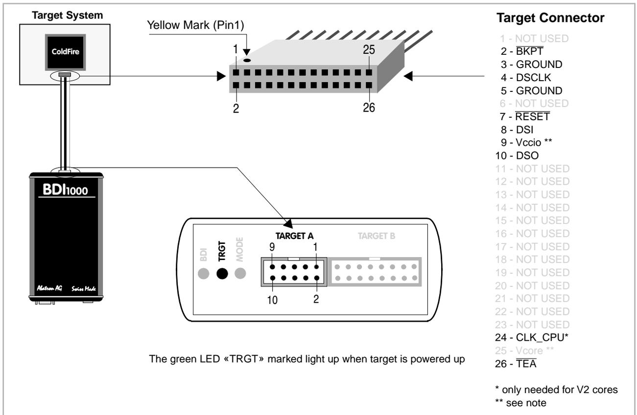
The target CPU clock is only needed for older V2 cores (MCF5204, MCF5206(e) and MCF5272) because DSCLK and DSI have to change synchronous with the CPU clock. For all other cores, BDM communication can be asynchronous to the CPU clock and therefore this signal is not needed.
