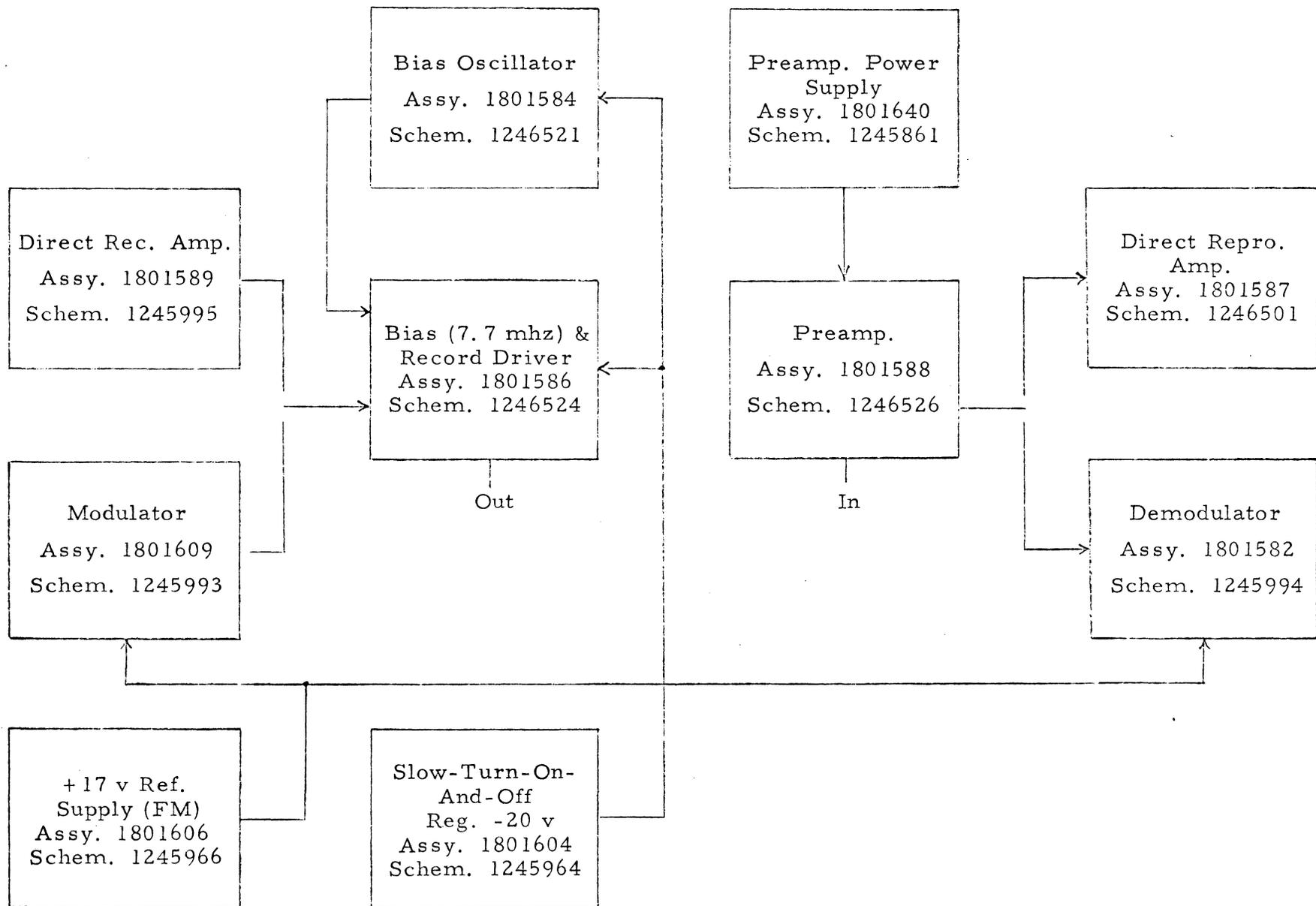
Figure 1. ES-200 System Block Diagram
