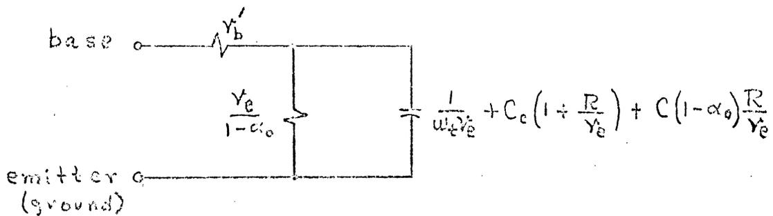
Figure 7. Equivalent Circuit of Input Impedance of Common Emitter Stage Q1.
