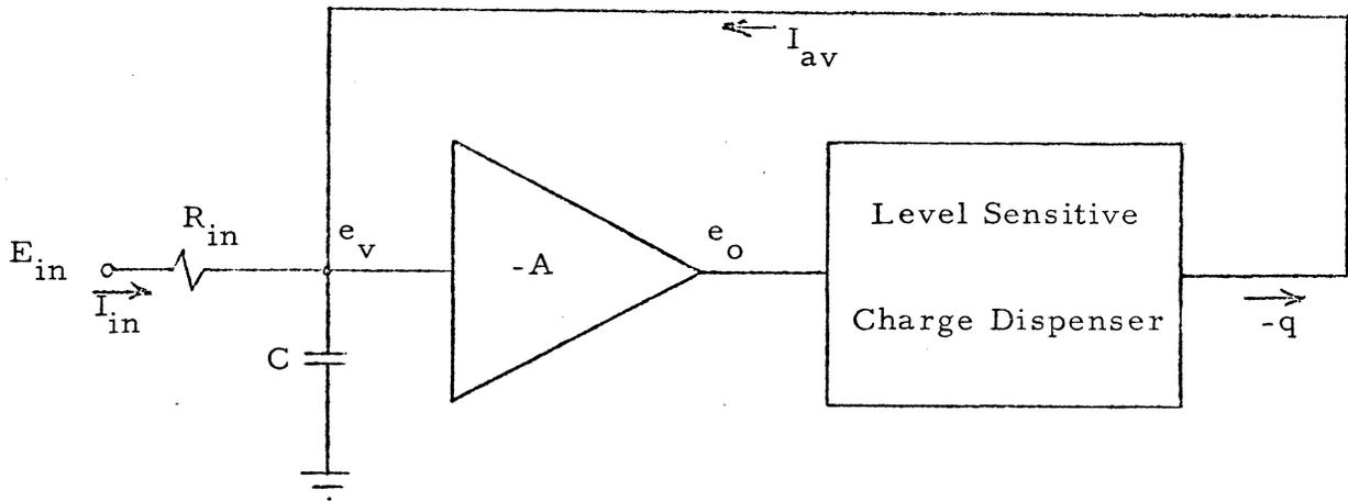
Figure 30a. Simplified Block Diagram of Modulator
