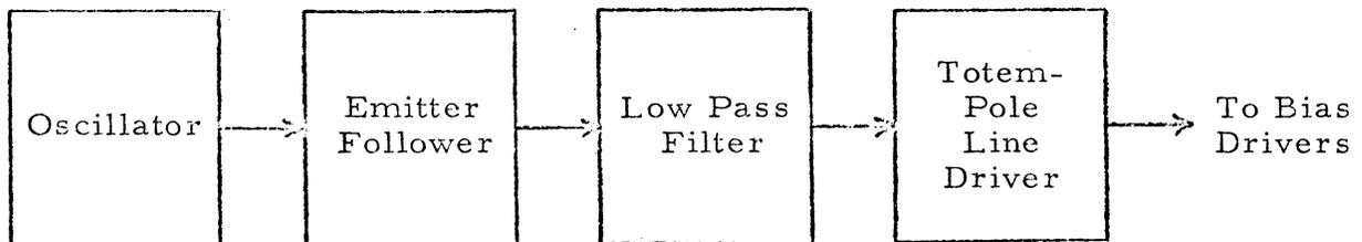
Figure 3. Bias Oscillator Block Diagram
