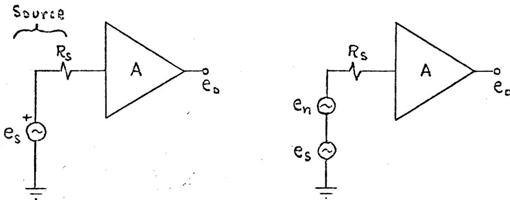
Figure 15. Noise Figure Block Diagram
