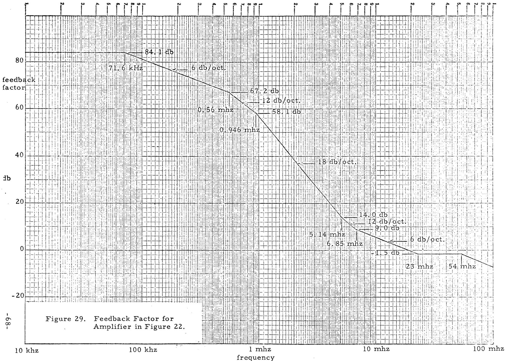
Figure 29. Feedback Factor for Amplifier in Figure 22.
