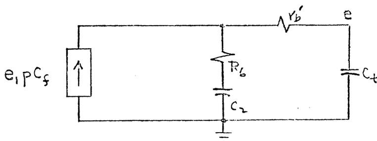
Figure 26. Modified First Stage Equivalent at 23 mhz
