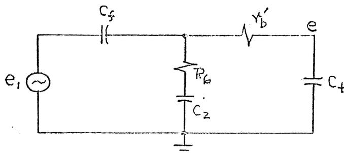
Figure 25. First Stage Equivalent at 23 mhz
