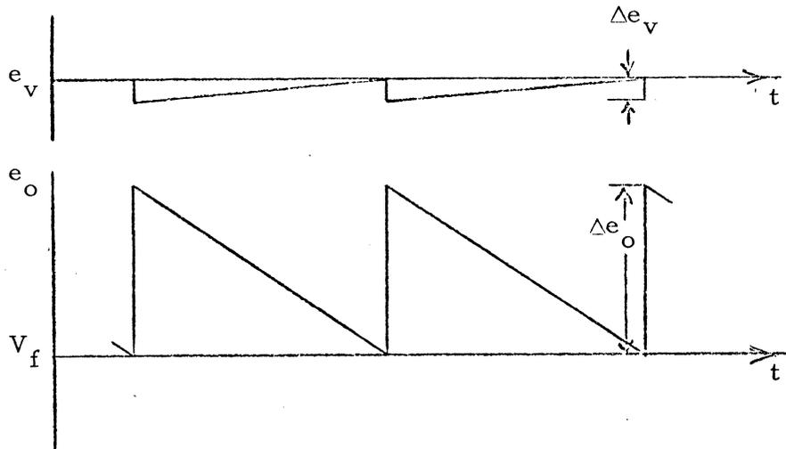
Figure 30b. Waveforms in Block Diagram of Modulator
