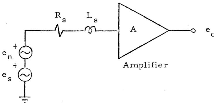
Figure 18. Series Noise Equivalent Circuit of Head and Preamp.
