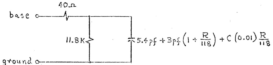
Figure 8. Equivalent Circuit of Input Impedance of Common Emitter Stage Q1.
