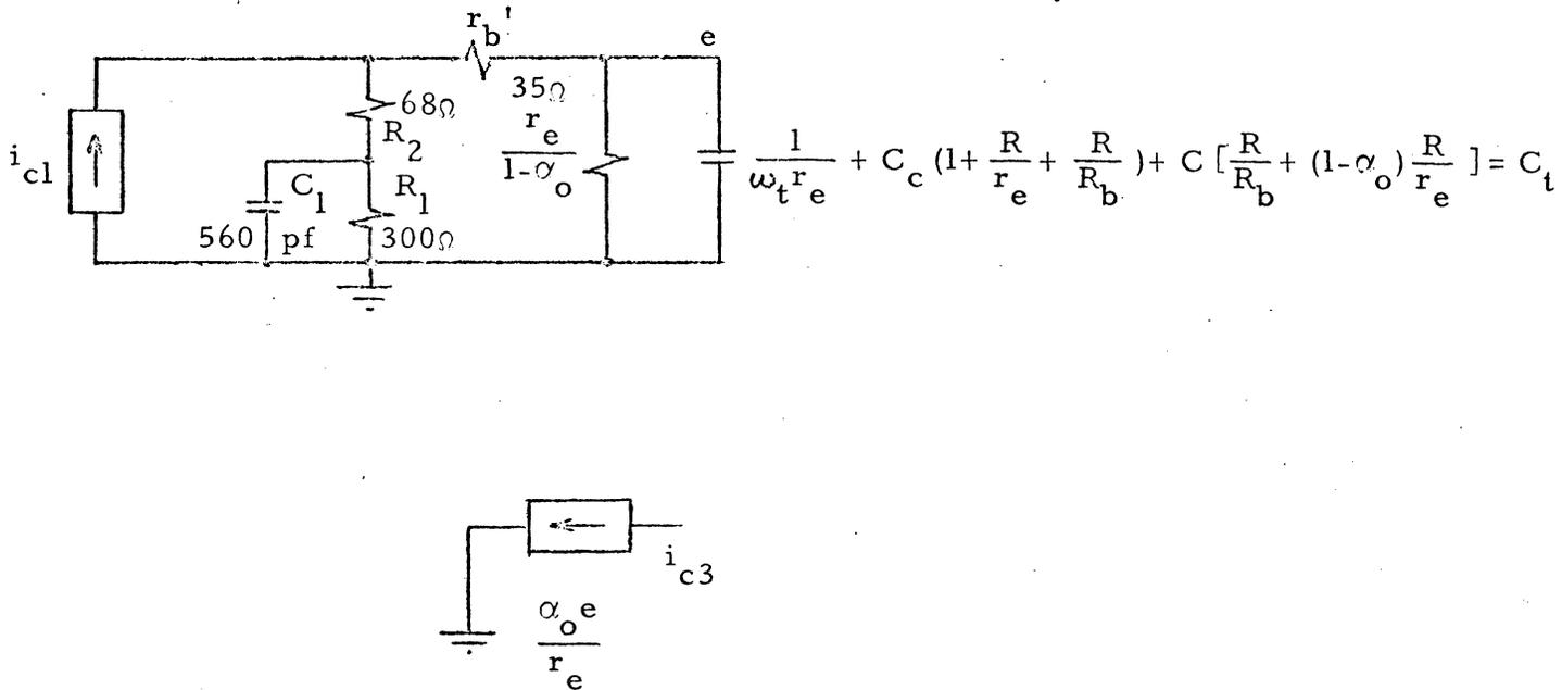
Figure 28. Equivalent Circuit of Q3.
