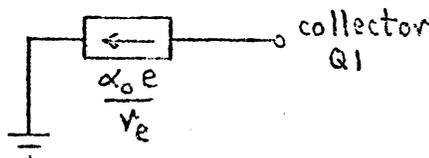
Figure 24. Equivalent Circuit for Feedback and First Stage
