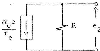
Figure 27. Equivalent Circuit of Q4.
