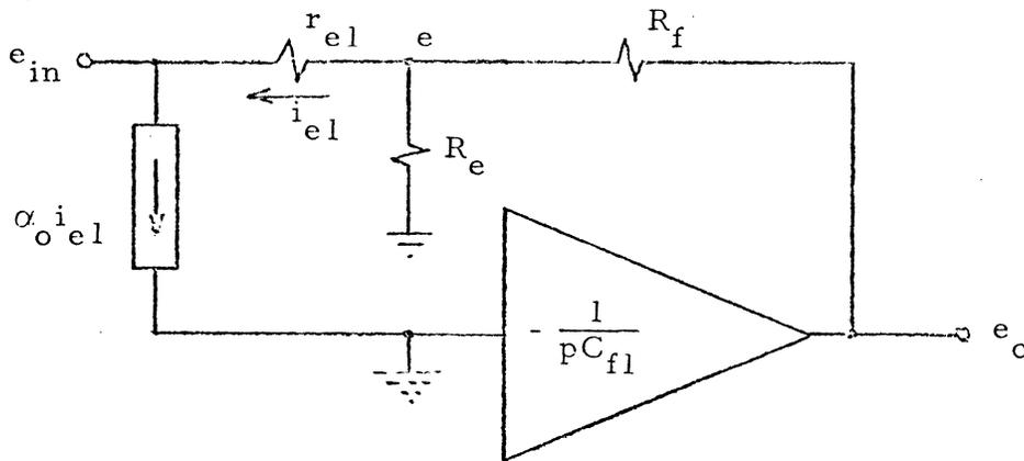
Figure 11. Equivalent Circuit of Amplifier
