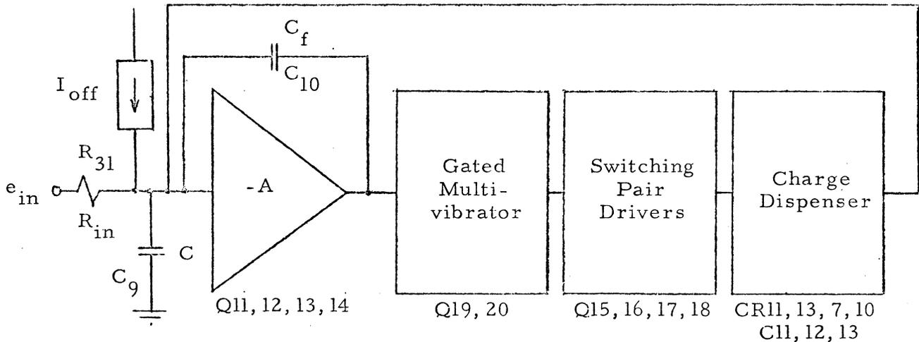
Figure 31. Block Diagram of Modulator
