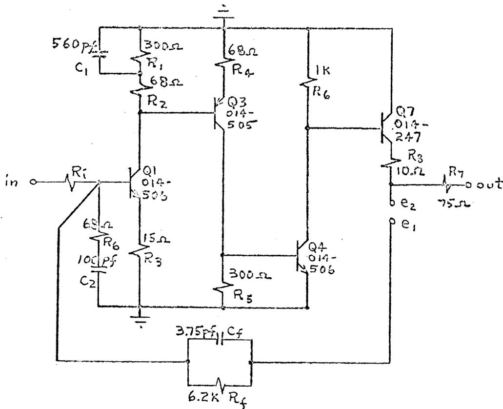
Figure 23. High Frequency Equivalent Circuit of Shunt Feedback Triple
