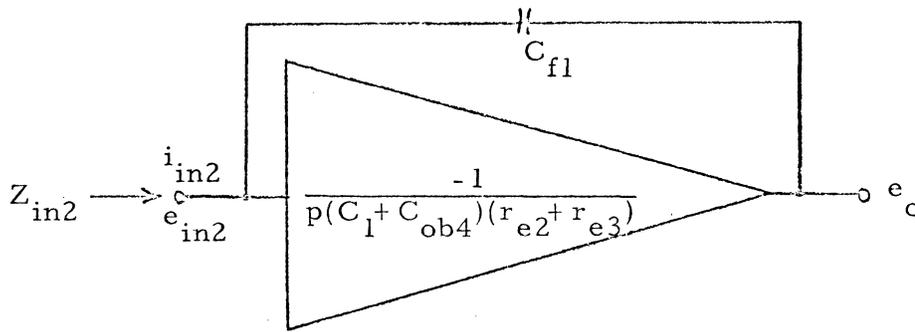
Figure 10. Equivalent Circuit for Q2, 3, 4, 5, and  $C_{f1}$ .
