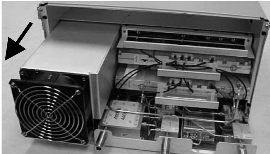
**Figure 7-6.** PDU Removal
