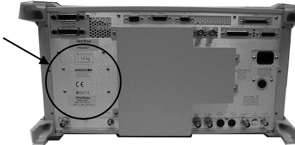
**Figure 7-13.** Option and Source Module Mounting Screws
