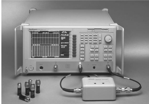
**Figure 7-2.** Two-Port AutoCal System Setup
