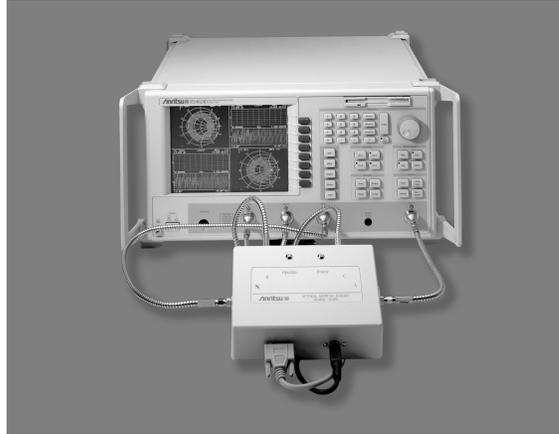
**Figure 7-3.** Four-Port AutoCal System Setup
