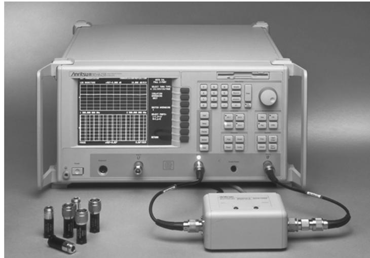
**Figure 3-1.** MS462XX with Two-Port AutoCal Module
