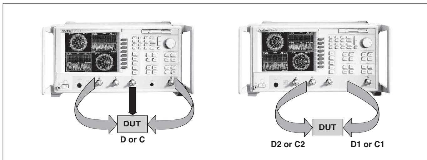
Measurement of 3 and 4-port single ended S-parameters are required in order to perform the mixed-mode conversion, which generates results as if the ports were being driven in pairs.
