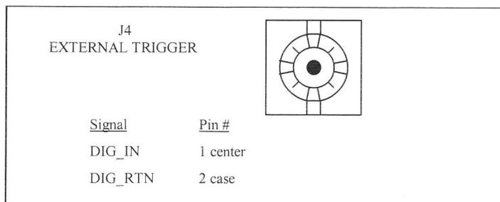
**FIGURE 8 - External Trigger Connector Diagram**
