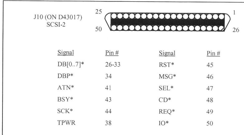
**FIGURE 7 - Optional SCSI-2 Connector Diagram**
