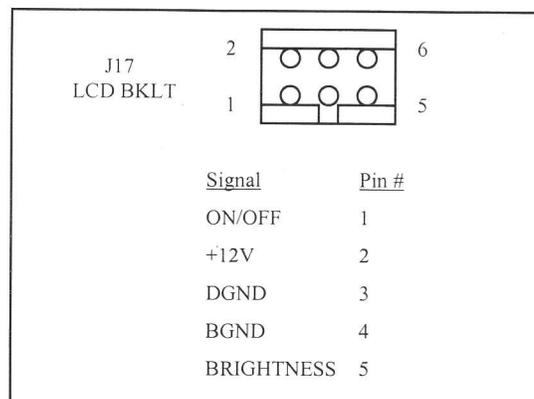
**FIGURE 12 - LCD Backlight Connector Diagram**
