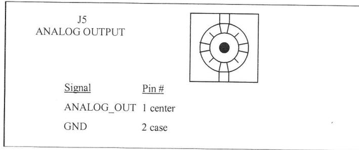
**FIGURE 9 – Analog Output Connector Diagram**
