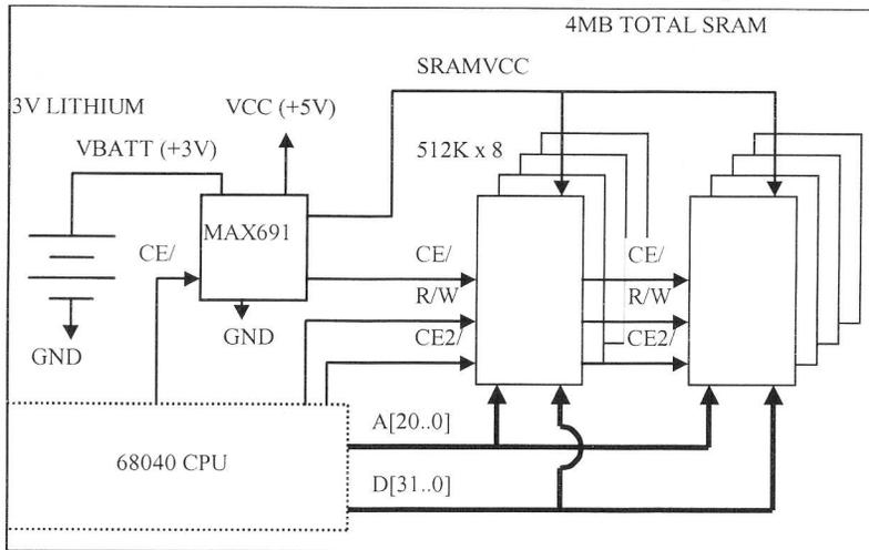
FIGURE 16 - Battery Backed SRAM
