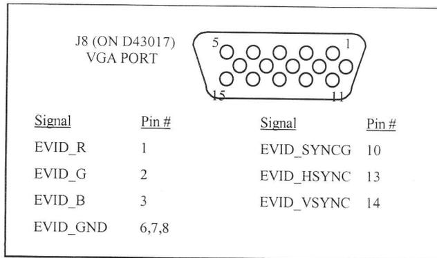
**FIGURE 6 - VGA Port Connector Diagram**
