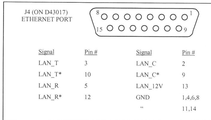
FIGURE 2 - Ethernet Connector Diagram
