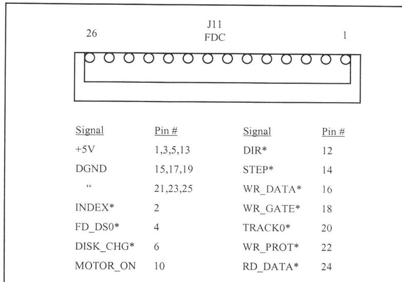
**FIGURE 14 - Floppy Disk Connector Diagram**
