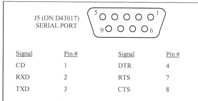
**FIGURE 5 - Serial Port Connector Diagram**
