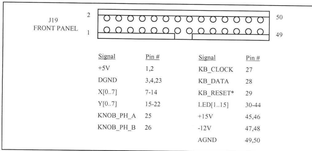
**FIGURE 13 - Front Panel Connector Diagram**
