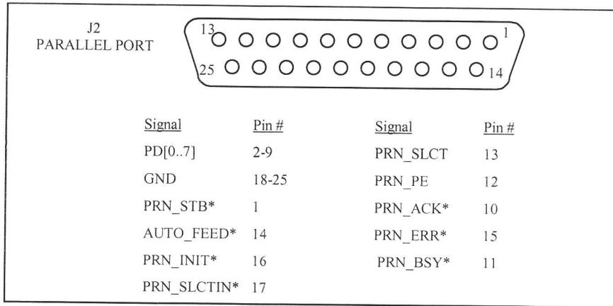
**FIGURE 4 – Centronics Printer Connector Diagram**
