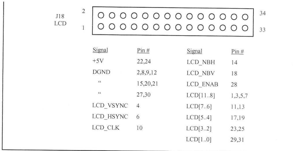
**FIGURE 11 - LCD Connector Diagram**
