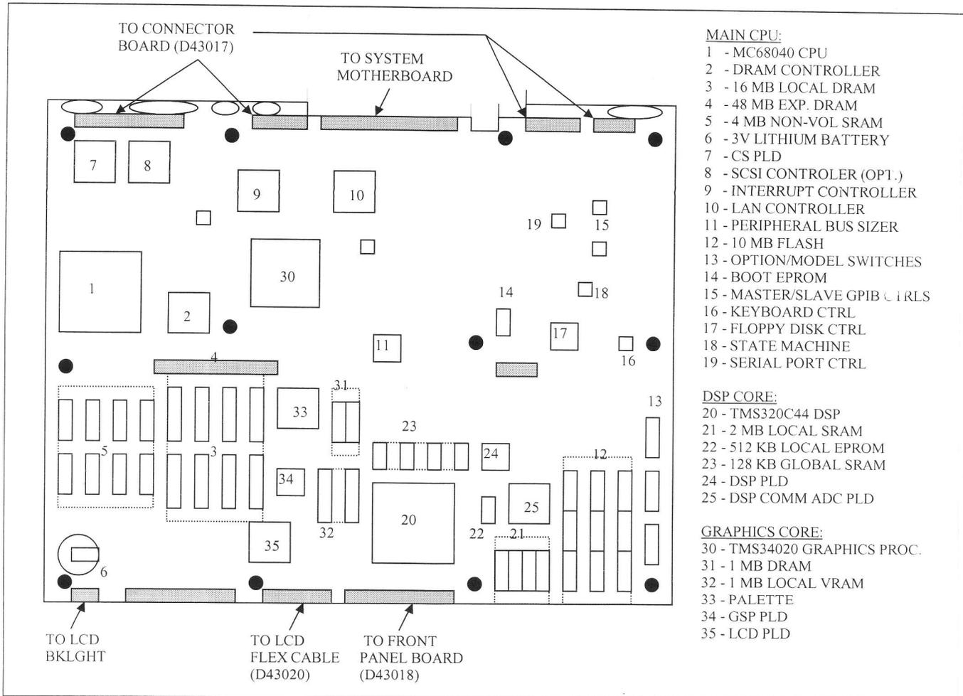
**FIGURE 1 - CPU Board Block Diagram**
