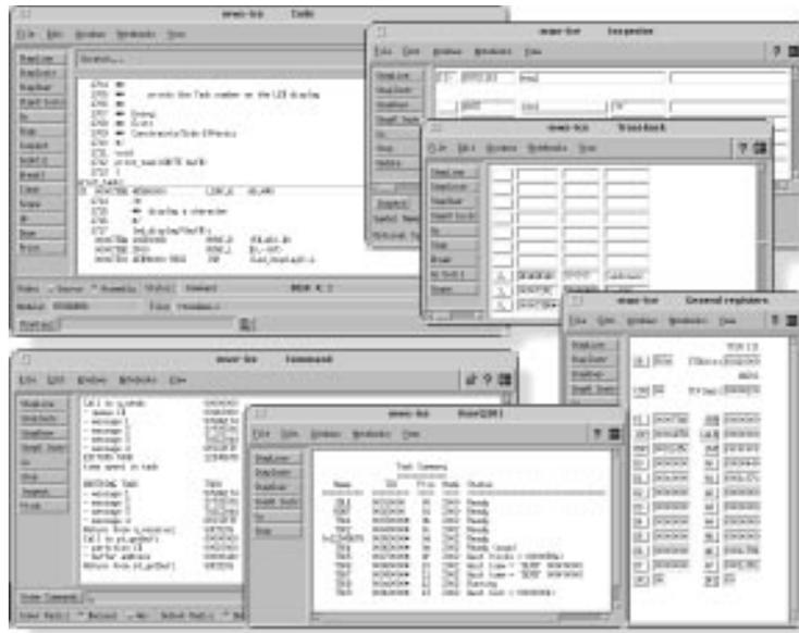
*The multi-windowed MWX-ICE debugger speeds development with simultaneous display including (clockwise from upper left): symbolic representation of structure elements; stack values; call tracing; register values; interleaved source and assembly; and pure source code.*
