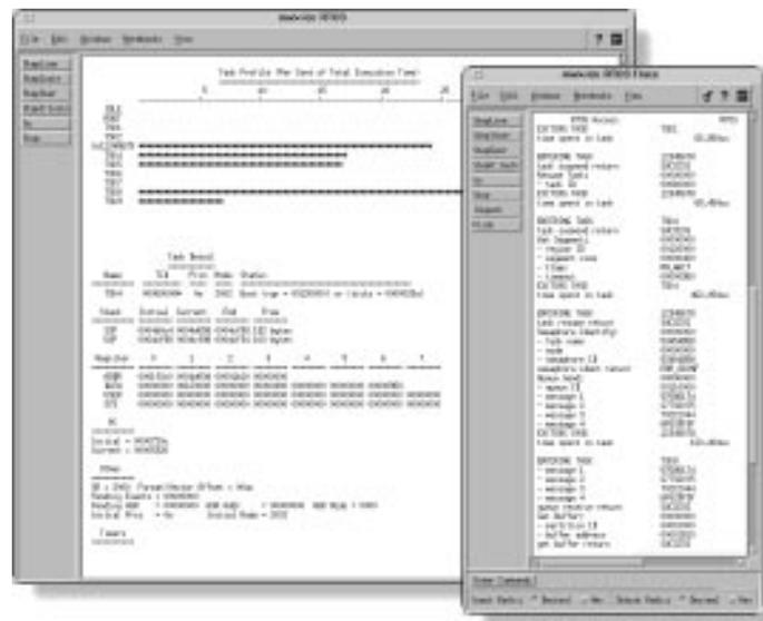
*RTOS-Link provides visibility of configuration and activities in kernel-based systems. Views such as task execution trace, task profiling, and configuration detail help you quickly isolate even subtle system problems.*
