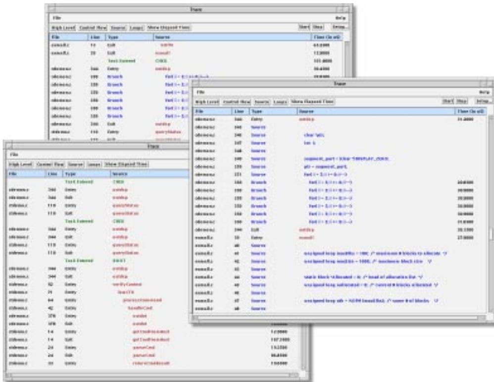
Program trace can be displayed in “high-level” mode where only task activity and function entries and exits are shown.
