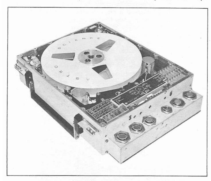
speeds of 1% through 60 ips and are available in 14 or 28-track configurations with 1 MHz at 60 ips wideband direct recording capability; or in 42-track configurations with 250 kHz at 60 ips direct recording capability. Digital recording is 1000 bits per inch per track. FM electronics are also available for intermediate band and wideband applications.
