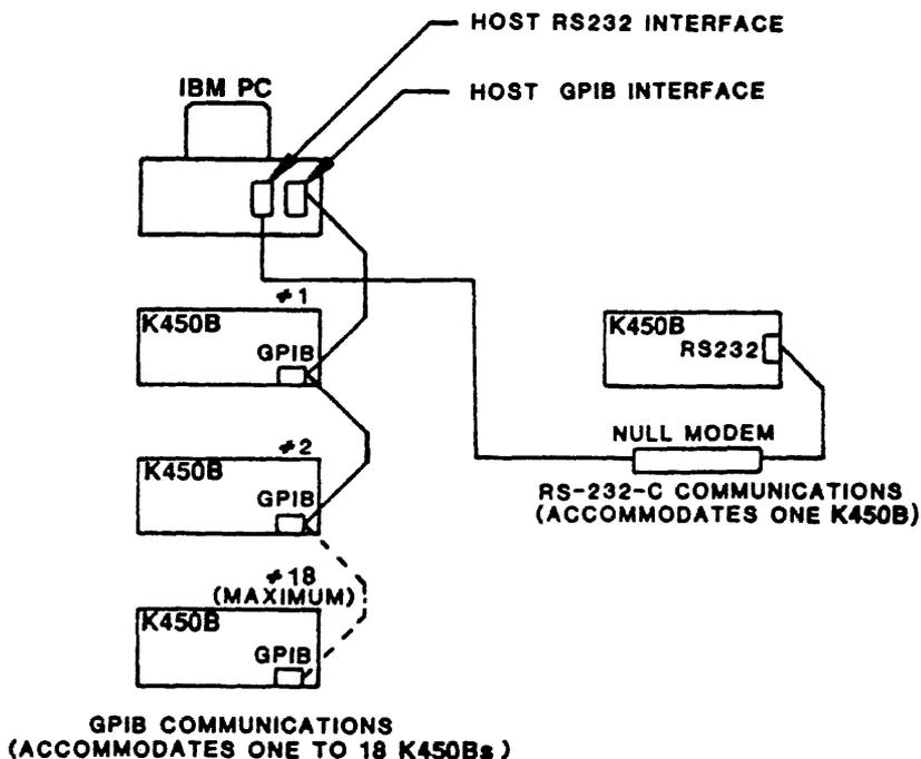
**Figure 1-1. PC Equipment Connections**
