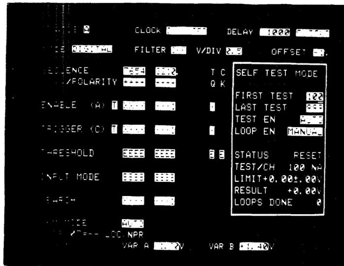
**Figure 3.3.3** Press the SELF-TEST key to obtain the self test display. The display will indicate which tests were failed, if any. The Maintenance Section of the manual explains the test information and operation.
