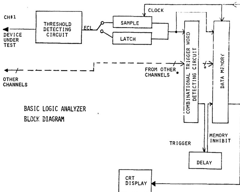
Figure 3.2.1 In order to better understand what is in the frozen data stream, a typical logic analyzer in block form is described here.
