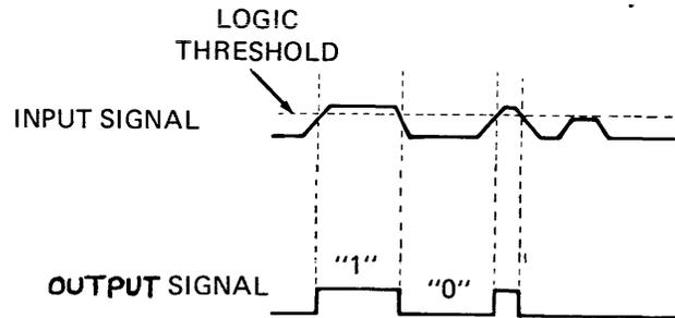
Figure 3.2.2 In the threshold detecting circuit, the input signal is compared to a selected logic threshold.
