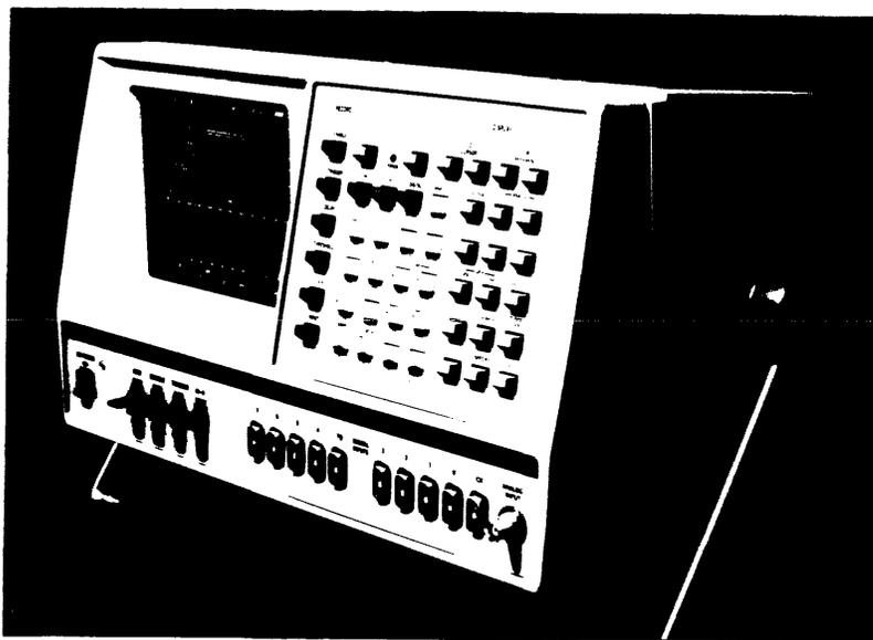
Figure 1.1 The Model K500-D Logic Analyzer is a technological breakthrough in logic analysis, with 500 MHz clocking, 2000 word memory, 8 digital signal inputs, an analog waveform digitizer input, unique scroll acquisition mode, and comprehensive time and data domain analysis facilities.
