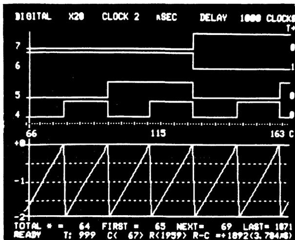
Figure 3.3.30 Digital and Analog recordings are displayed simultaneously.
