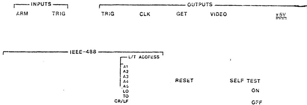
**Figure 3.3.31** The 8 in-line DIP switch labeled L/T address select the bus address, the mode and line terminator. When the switch is down on the side marked open, it is a zero. Switches A1 through A5 are the address switches with A1 as the LSB.
