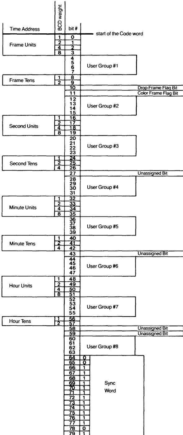
Figure 6 — TIME CODE DATA STRUCTURE
