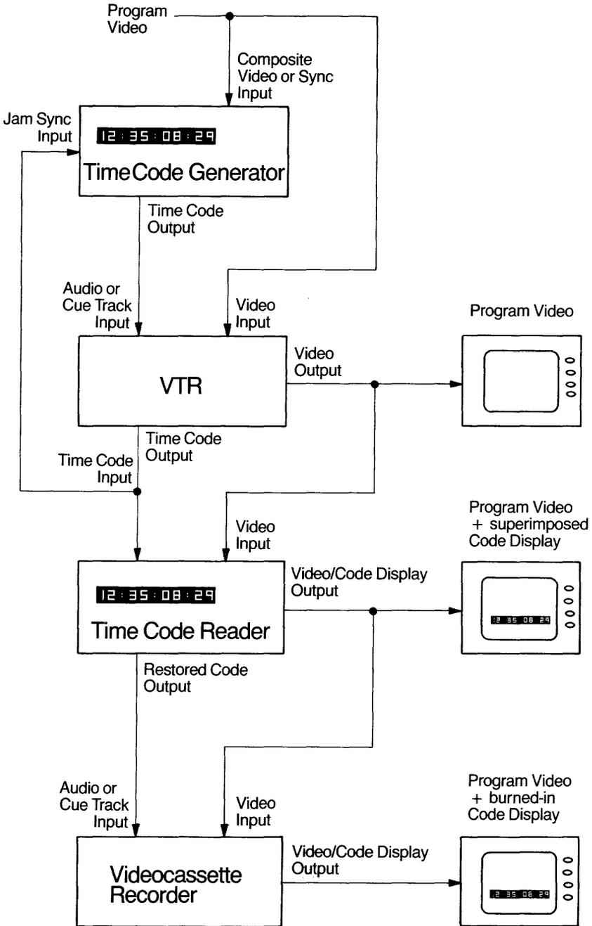
Figure 4 — SYSTEM DIAGRAM
