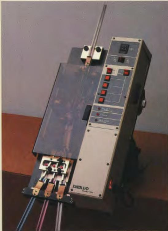
**DESIGNED TO QUICKLY HANDLE STANDARD DEVICE PACKAGES.** The Handler 300 has been designed to accommodate standard 6- to 24-pin lead DIP devices with 300 mil bend centers. To handle 28- to 40-pin lead DIP devices with 600 mil bend centers, equip your production programmer with the Model 600. Both the 300 and 600 handle up to 8,000 devices per hour at zero test time. In addition, they incorporate a programmable three-sleeve sort which allows you to differentiate between failed devices.
