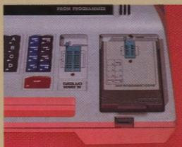
One of several hardware options available for the Series 22 is a "smart adapter" containing built-in firmware to change the prompting parameters for programming application-
