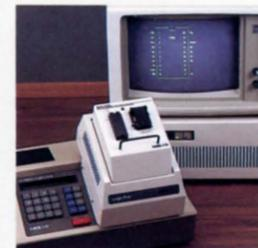
Link the PLDS with a personal computer to facilitate logic design and programming.
