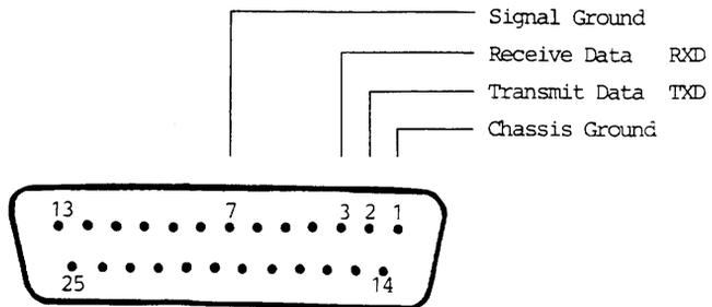
Figure 5-1: Standard RS-232-C Pinout
