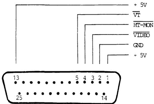
Figure 3-11: Video Interface Pinout
