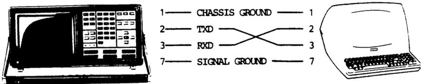
Figure 5-2: Line Connection Example
