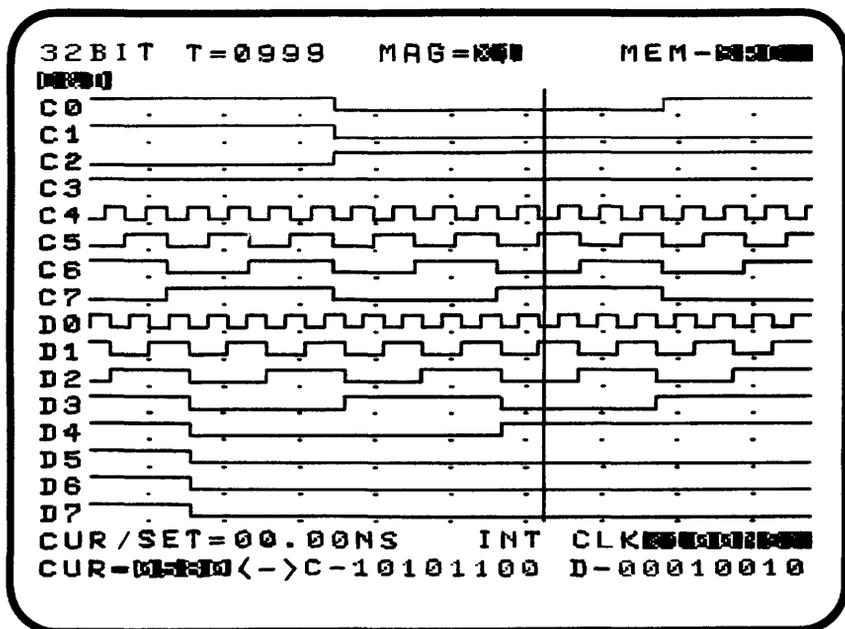
Figure 4-16: Timing Diagram
