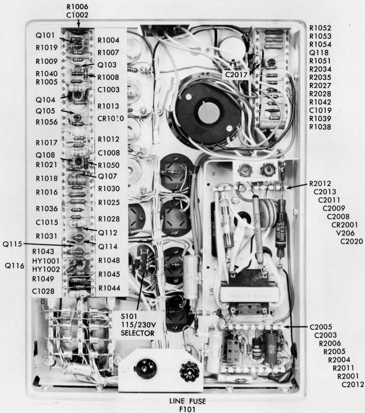
FIGURE 3-4. IDENTIFICATION OF REPLACEABLE COMPONENTS ON REAR CHASSIS
