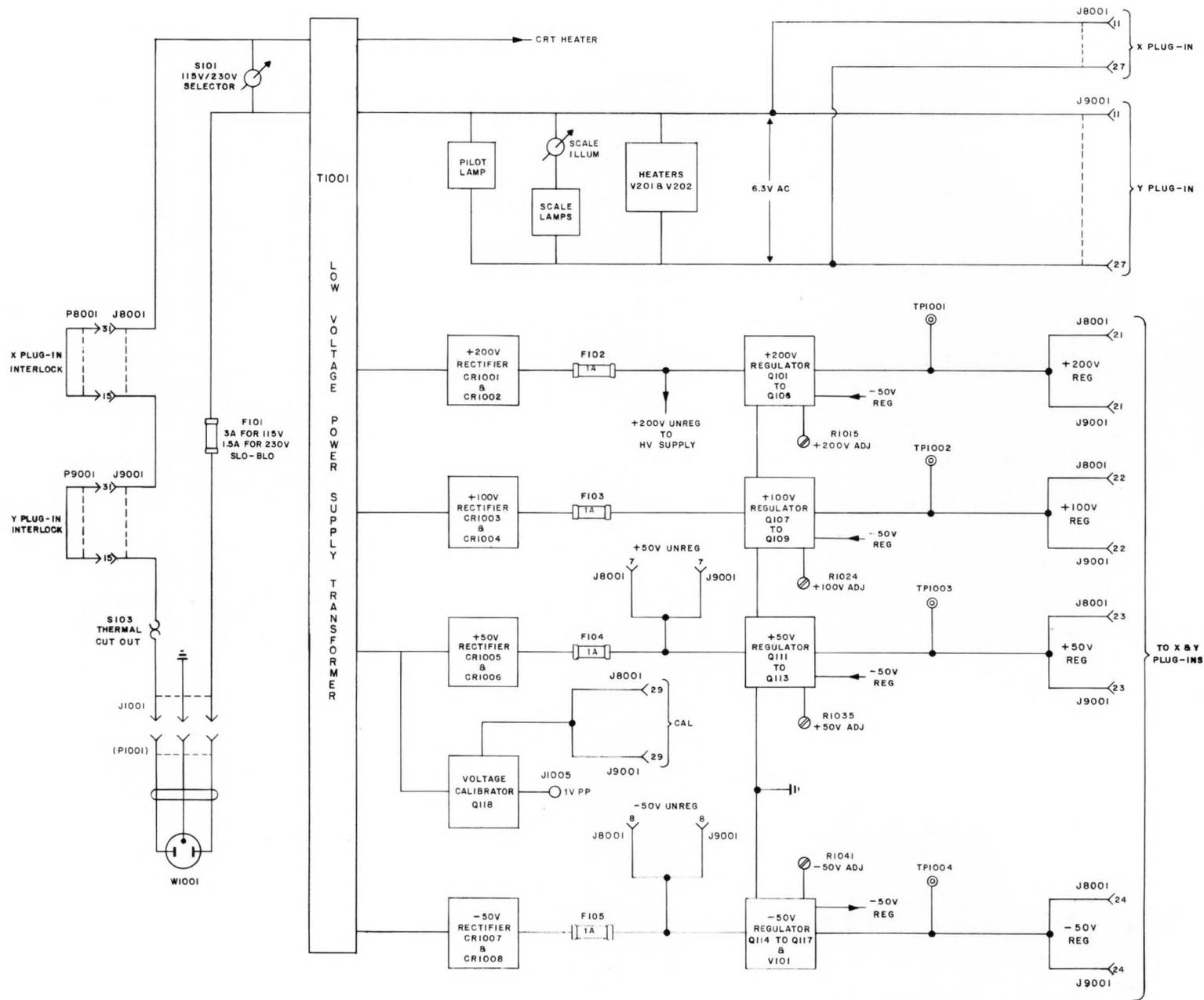
FIGURE 3-1. MAIN FRAME LV POWER SUPPLY FUNCTIONAL BLOCK DIAGRAM
