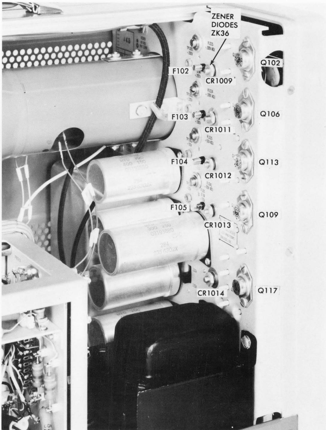
FIGURE 3-3. IDENTIFICATION OF REPLACEABLE PARTS (RIGHT SIDE VIEW)
