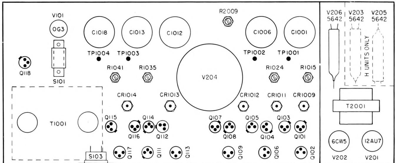
FIGURE 3-6. LOCATION OF COMPONENTS FOR RACK AND PORTASCOPE MODELS (REAR VIEW)
