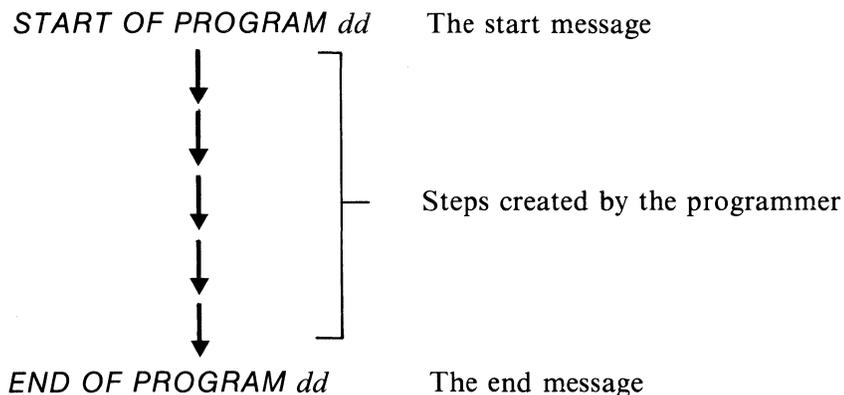
The start message and end message are only for reference when examining the program as it is stored in the 9010A. The start message and end message are not part of the program listing that is transferred via **AUX I/F**, and do not appear when a program is printed out or viewed on a video display.
