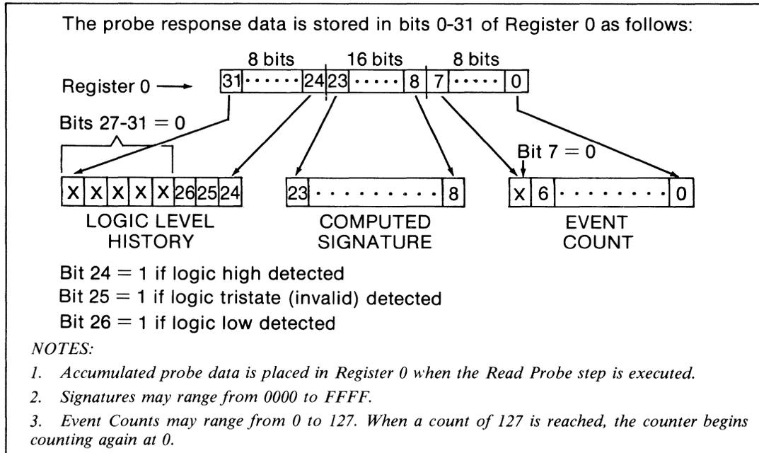
Figure 5-1. Probe Data Format for Register 0
