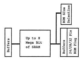
The slave module extends a given unit's capacity to emulate two ROMs. The maximum capacity of a unit equipped with a slave module is thus 2 mega bytes or 16 mega bits!
