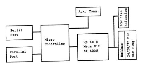
The product is based on an intelligent micro controller (Signetics 87C451) communicating with the host processor (PC etc.) over the RS-232C serial link or the parallel link. The emulator is connected to the ROM socket on the target via a ribbon cable. The auxiliary connector provides a programmable 'reset' and other signals for target control
