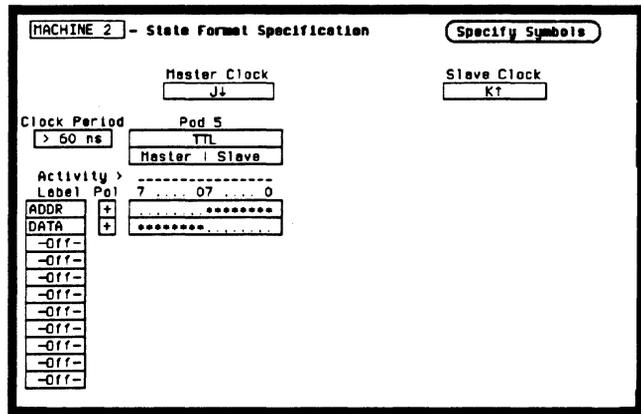
**Figure 9-13. Master and Slave Clock Bit Assignments**
