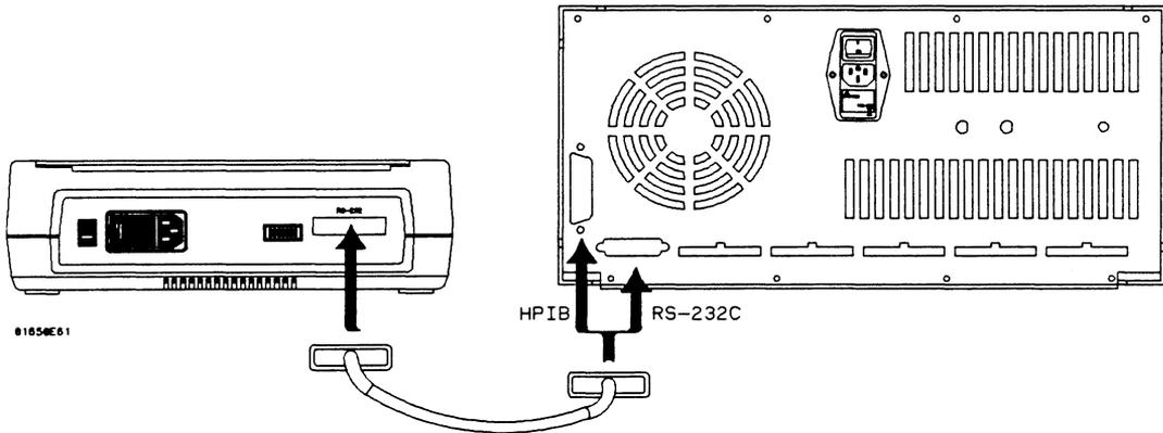
**Figure 7-1. Logic Analyzer to Printer Hook-up**
