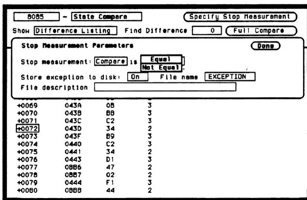
Figure 12-4. Specify Stop Measurement Field
