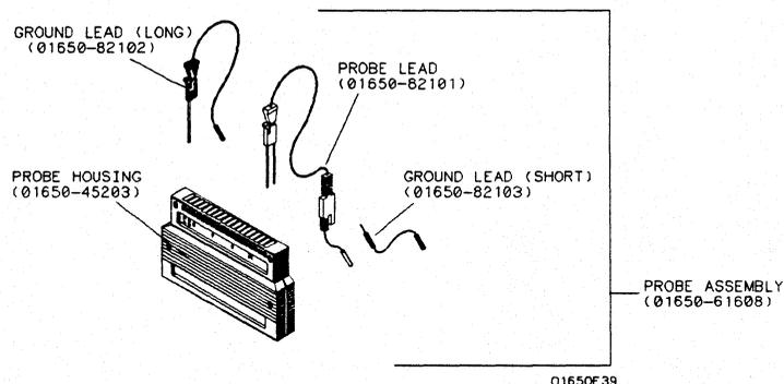
Figure 2-3. Probe Assembly
