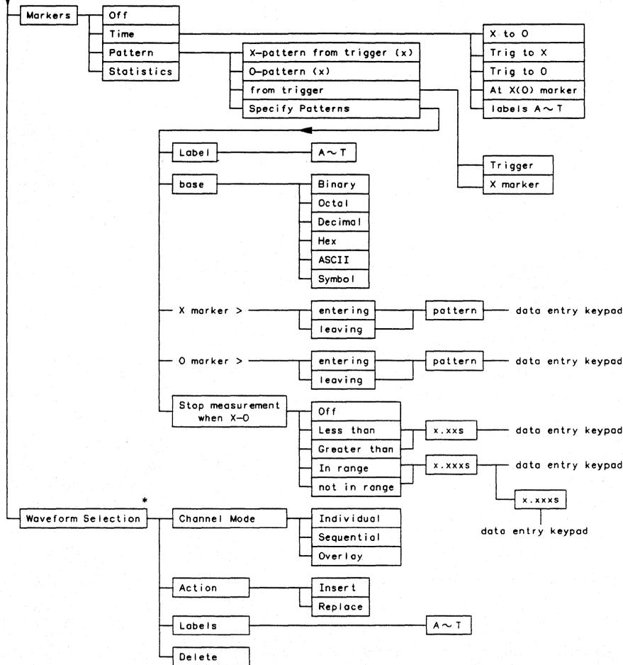
\*Access by touching the box on the far left of the waveforms display where the labels are displayed
