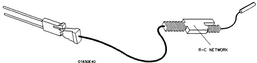
Figure 2-4. Probe Cable
