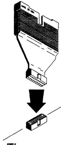
Figure 2-2. Termination Adapter
