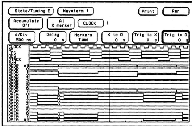
Figure 6-2. Timing Waveforms Menu with 24 Waveforms
