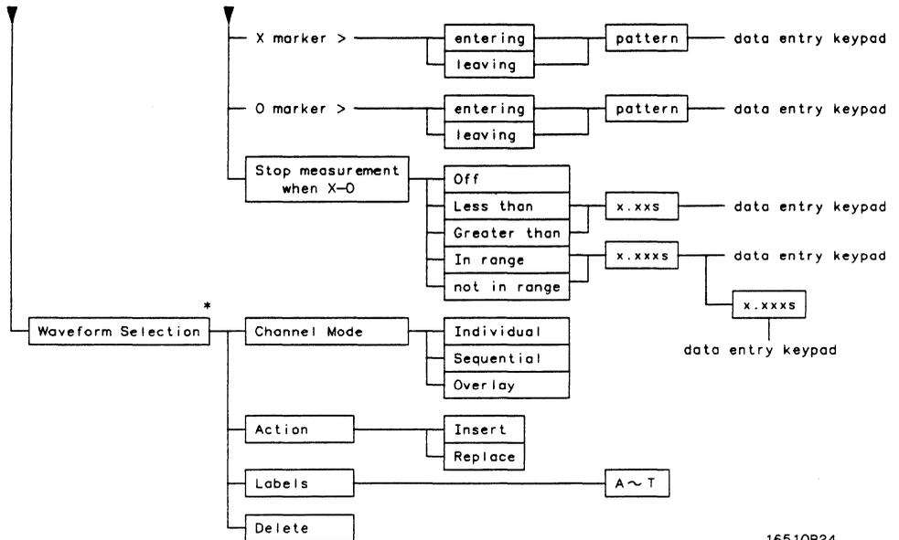
\*Access by touching the box on the far left of the waveforms display where the labels are displayed
