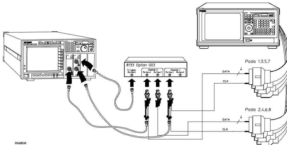
Connect the HP 1662C/CS/CP or HP 1663C/CS/CP Logic Analyzer to the Pulse Generator
