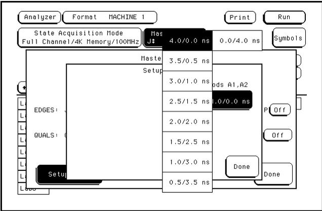
**e** Select the field to the right of the pod being tested, then select TTL.
