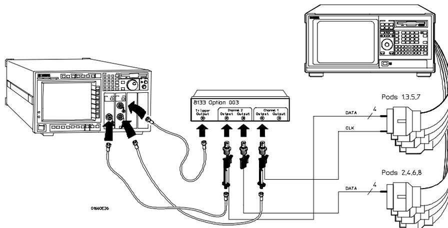
Connect the HP 1662C/CS/CP or HP 1663C/CS/CP Logic Analyzer to the Pulse Generator
