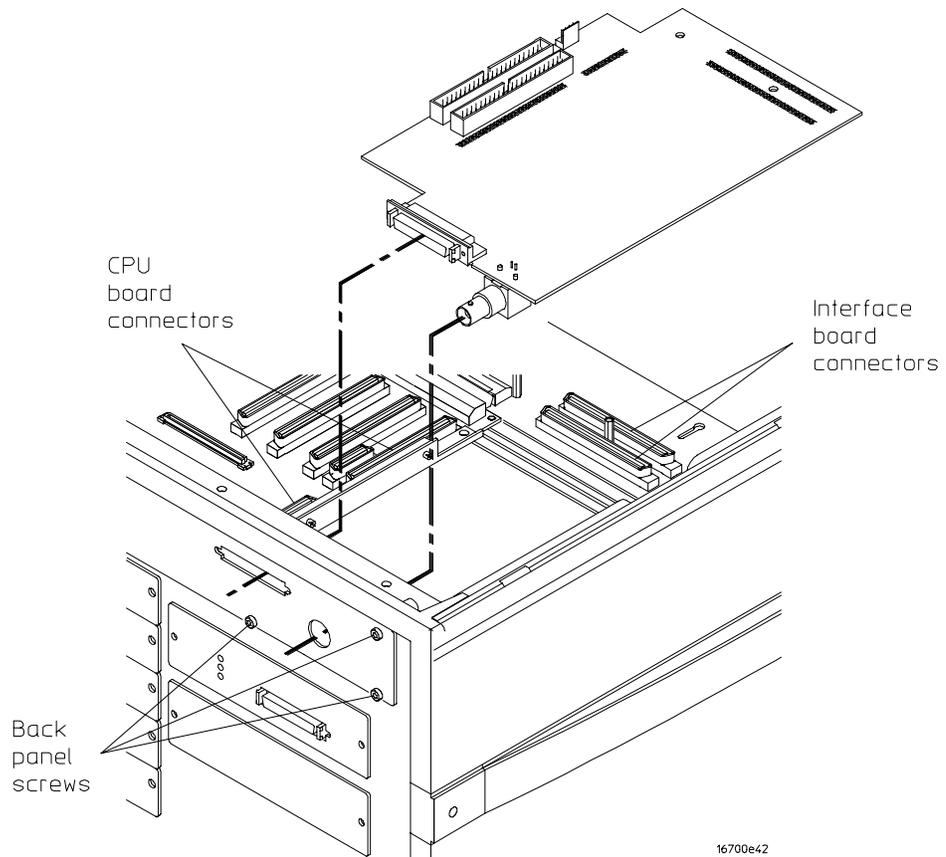
**7 Reverse this procedure to install the PCI board. Before installing the PCI board, ensure that the following assemblies are properly installed:**
