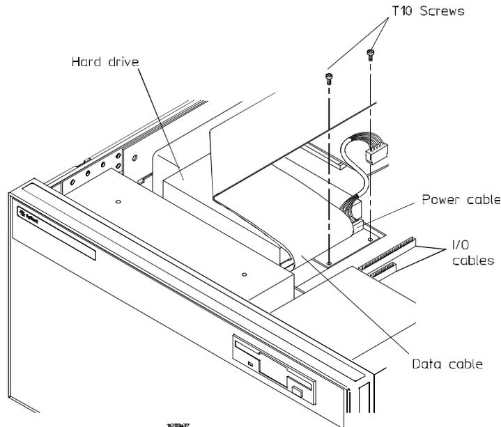
**4** Using a Torx T10 screwdriver, remove the two screws that secure the hard disk drive bracket to the frame (see the preceding illustration).
