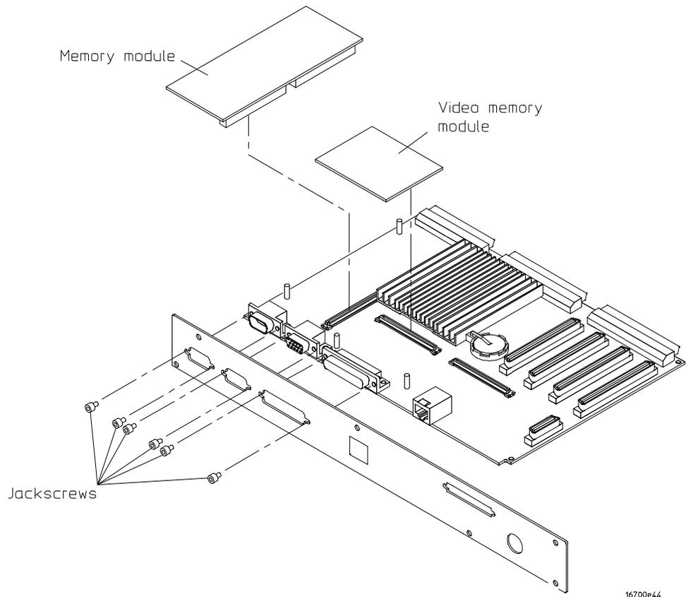
**5** Exchange System RAM and Video RAM (if installed) between the defective and replacement CPU boards.
