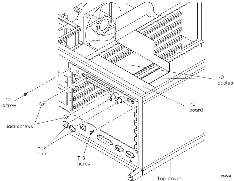
**3** Using a Torx T10 screwdriver, remove the two screws that secure the I/O board to the rear panel.
