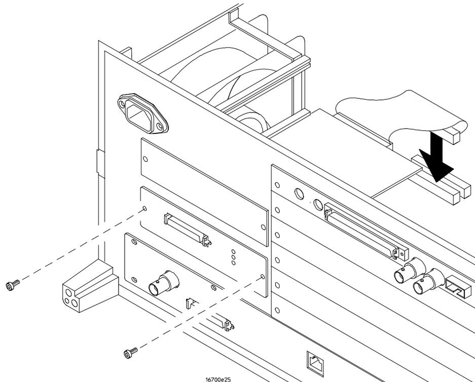
**4** Slide the emulation module out the rear of the instrument.
