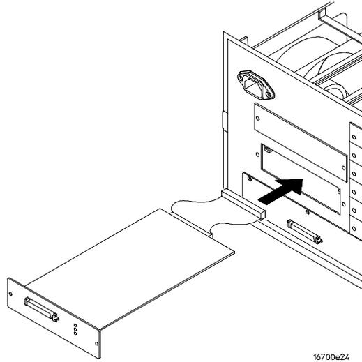
**7** Connect the cable and re-install the screws.
