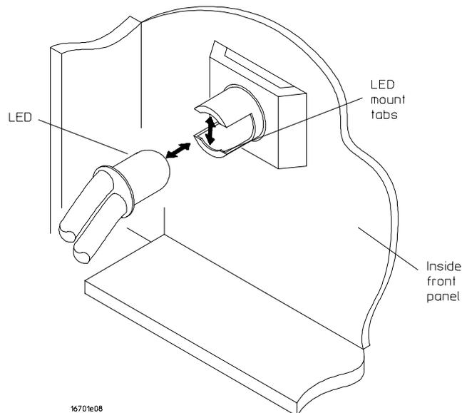
**3** To install the LED, position the LED onto the mount and gently apply force until LED snaps into the mount. A little gentle wiggling of the LED will help the process along, too.
