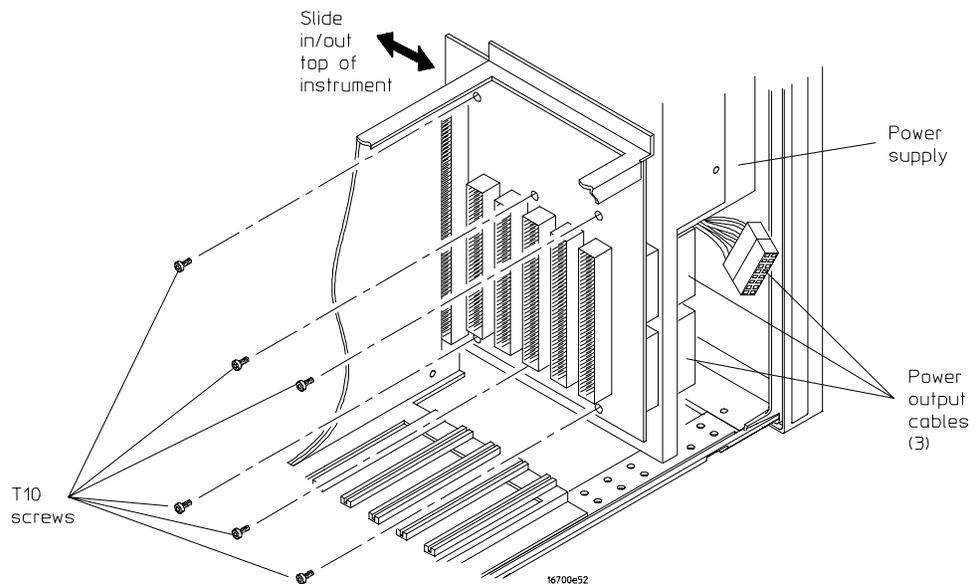
**5** Remove the module interface board out the top of the instrument.
