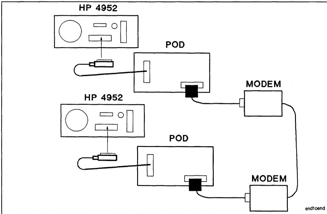
Figure 10-4. End-to-End Testing
