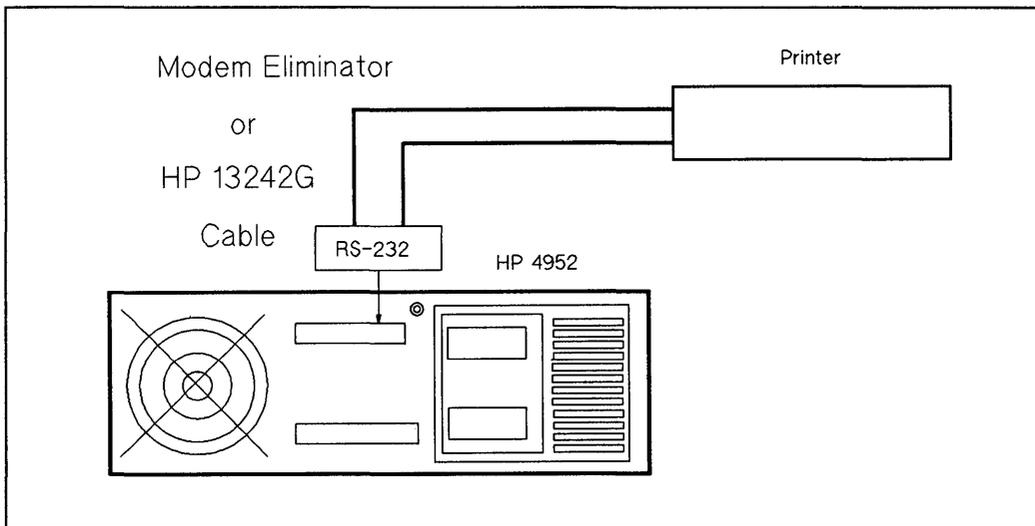
**Figure 13-1. Connecting the Printer**
