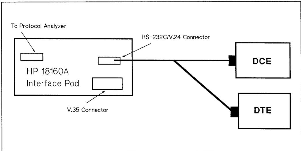
**Figure 15-7. RS-232C/V.24 Pod Configuration - Monitor Mode**
