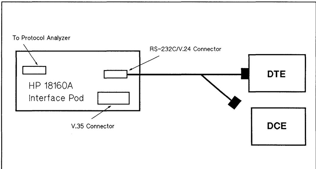
**Figure 15-9 RS-232C/V.24 Pod Configuration - Simulating a DCE**
