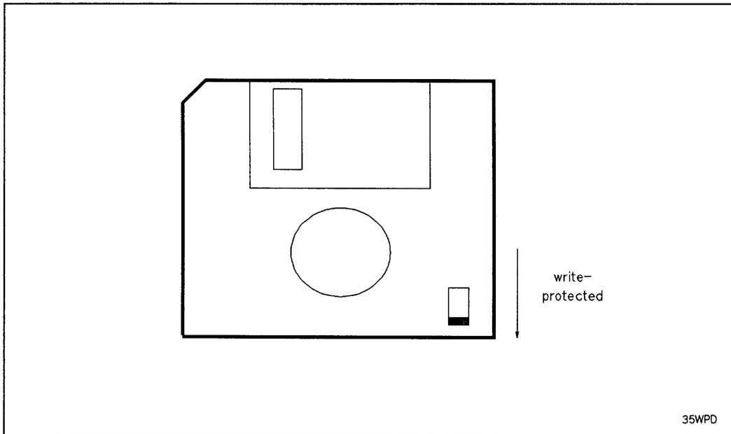
**Figure 12-2. Write Protecting Your Disc**
