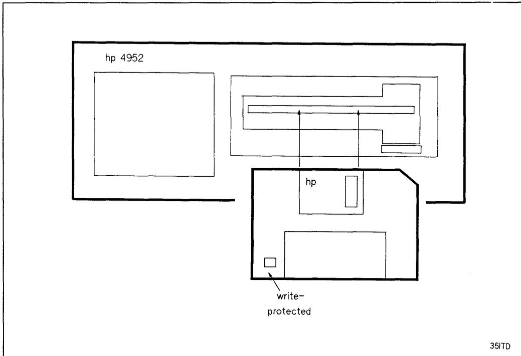
**Figure 12-1. Inserting the Disc**
