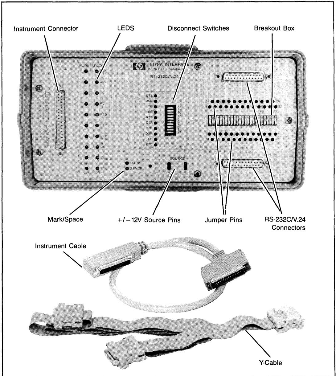
**Figure 1-3. The HP 18179 Interface Pod**
