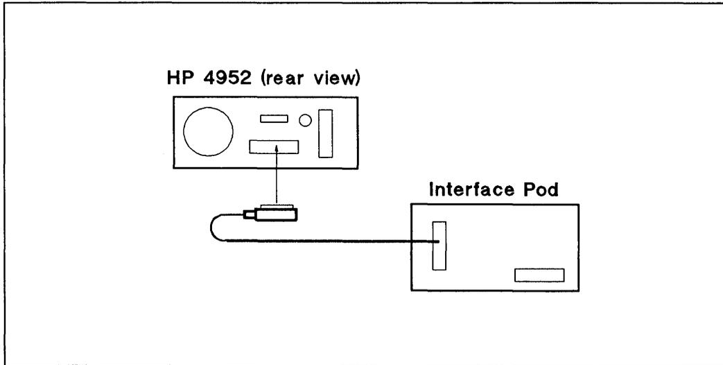
**Figure 15-1. Interface Pod Connection**
