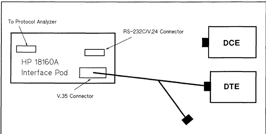
**Figure 15-11 V.35 Pod Configuration - Simulating a DCE**
