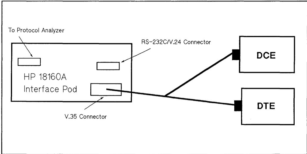
**Figure 15-10. V.35 Pod Configuration - Monitor Mode**
