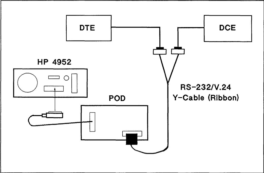
Figure 4-1. Hookup for Monitoring the Line
