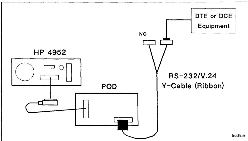
Figure 7-1. Hookup for Simulating
