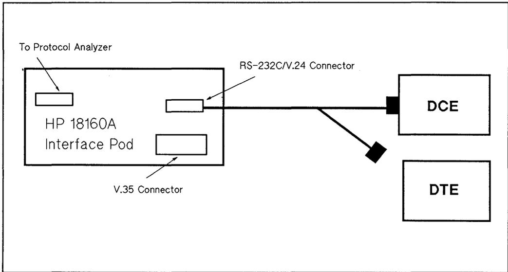
**Figure 15-8 RS-232C/V.24 Pod Configuration - Simulating a DTE**
