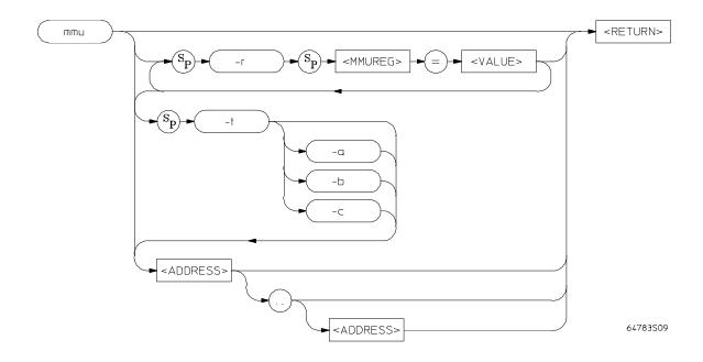
The **mmu** command is used to display valid logical-to-physical address translations. You can display the present translations for all logical addresses, or for only a limited range of logical addresses. Further, you can display the details of how a single logical address is mapped through the tables to its corresponding physical address. Finally, you can display the details of a single translation table used by a selected logical address.
