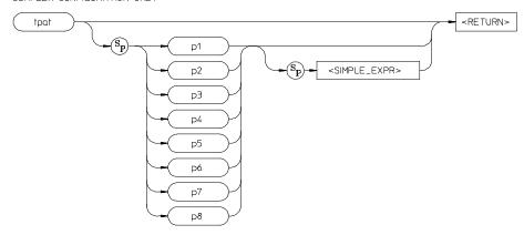
The **tpat** command allows you to assign pattern names to simple analyzer expressions.
