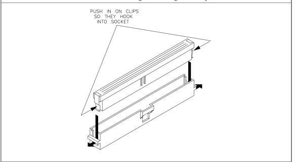
**3** Connect the other ends of the cables to the emulator probe. Again, make sure the stainless steel clips on the cable connectors are properly latched within the sockets, as shown in step 2.
