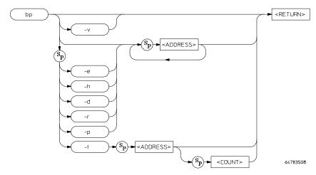
The **bp** command is used to insert, delete, display, or modify the status of execution breakpoints. Upon powerup or **init** initialization, the breakpoint table is cleared and the breakpoint feature is enabled. If no parameters are specified, the current status of all breakpoints is displayed.
