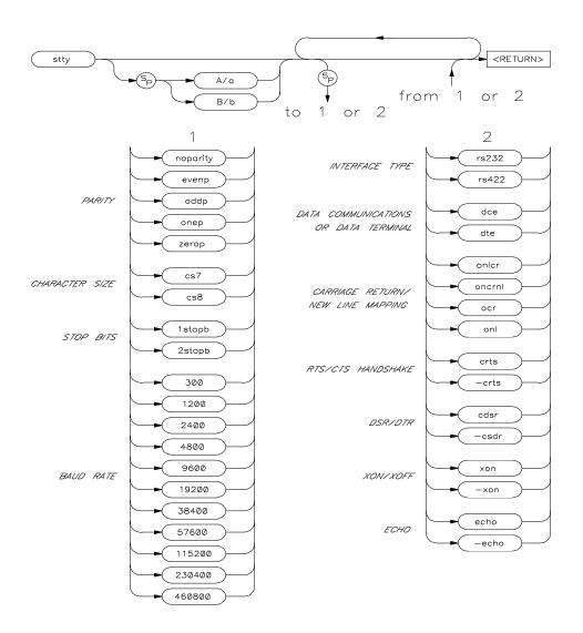
The **stty** command allows you to modify the parameters of the data communications ports without changing the configuration switch settings.
