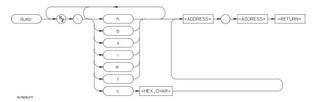
The **dump** command allows you to dump the contents of emulation and/or target system memory to a host file. The contents can be dumped in HP, Tektronix hex, Intel hex, and Motorola S-record formats by specifying various options on the command line.
