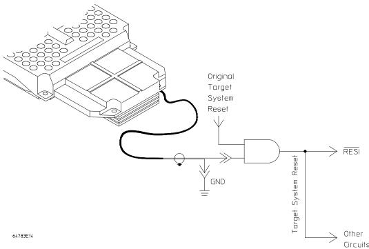
The example circuit shows the emulator reset signal being ANDed with a target system reset signal to generate a new target system reset signal. This new signal will reset the processor and other circuits on the target system when either the emulator asserts reset, or the target system generates reset.
