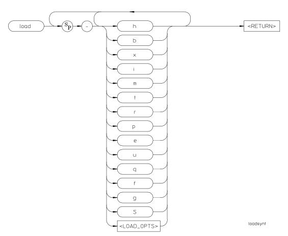
The **load** command lets you load program code into emulation or target memory. Various file formats are supported via options to the load command.
