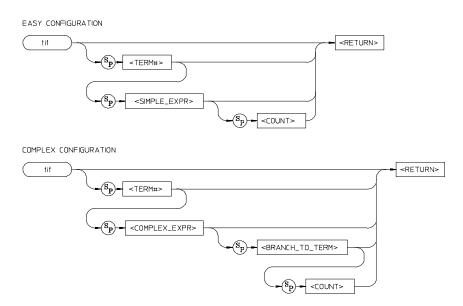
The **tif** command allows you to set the primary branch qualifier for each term of the emulation-bus analyzer sequencer.
