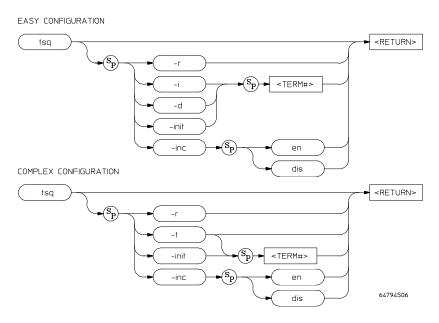
The **tsq** command allows you to manipulate or display the trace sequencer. Note that the **tif** and **telif** commands are used to define each sequencer state specification.
