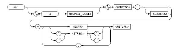
The **ser** command allows you to search memory for a data value, a character string, or a combination of both. For every pattern match, the starting address of the match is displayed.
