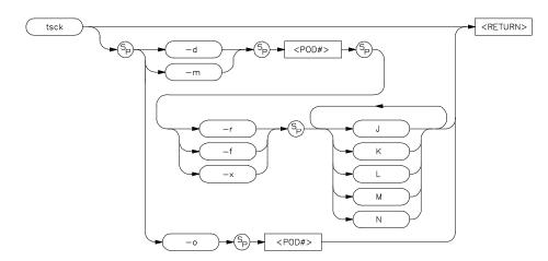
In the 1K analyzer, the **tsck** command allows you to specify the slave clock edges used for the emulation-bus analyzer trace. Slave clocks are not supported in the deep analyzer.
