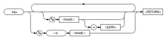
The **equ** command allows you to equate arithmetic values with names that you can easily remember; these names can then be used in other commands to reference the value. This is useful in defining trigger patterns for the analyzer and in other applications.
