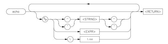
The **echo** command allows you to display ASCII strings or the results of evaluated expressions on the standard output device.
