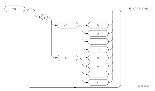
The **mo** command allows you to modify the global access and display modes. Access mode is defined as the type of processor data cycles used by the emulation monitor to access a portion of your memory. Display mode is defined as the method used to display or modify data resident in memory.
