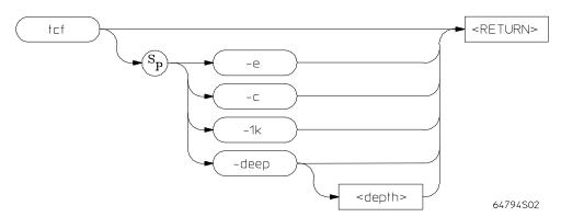
The **tcf** command is used to set the configuration for the emulation-bus analyzer. The **-1k** and **-deep** parameters are available only when using the deep analyzer.
