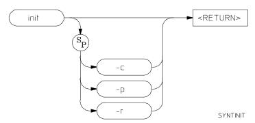
The **init** command allows you to reinitialize the emulator. Powerup, complete, and limited initializations are available through various options.
