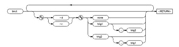
The **bnct** command allows you to specify which of the internal **trig1/trig2** trigger signals will drive and/or receive the rear panel BNC trigger. You can specify the signals individually, as an ORed condition for drive, or as an ANDed condition for receive; or, you can specify that the signals are not to be driven or received.
