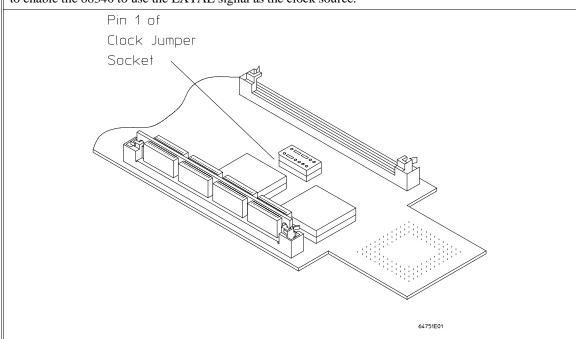
Chapter 2: Plugging into a Target System **Step 3. Select the emulator clock source**
