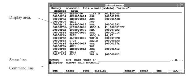
**Display area.** Can show memory, data values, analyzer traces, registers, breakpoints, status, simulated I/O, global symbols, local symbols, pod commands (the emulator's underlying Terminal Interface), error log, or display log. You can use the UP ARROW, DOWN ARROW, PAGE UP, and PAGE DOWN cursor keys to scroll or page up or down the information in the active window.
