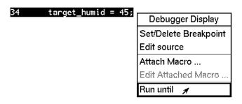
Line 34 should now be highlighted. Notice that "init\_system" now appears in the Backtrace window at level 0, which means that the program counter is inside the *init\_system()* function.
