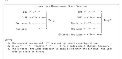
This display illustrates the possible connections between the internal lines (trig1 and trig2) and the emulator, analyzer, and external devices.
