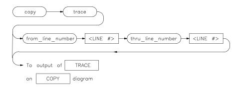
This command copies the contents of the trace buffer to a file or to the printer.
