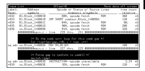
Notice in the resulting trace (you have to press the <NEXT> key) that the enable and disable states have the "sq adv" string in the line number column. This is because the windowing feature uses the analyzer's sequencer.
