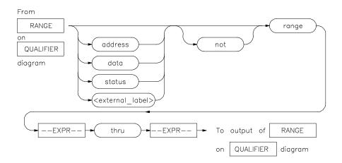
The **RANGE** parameter allows you to specify a condition for the trace measurement, made up of one or more values.
