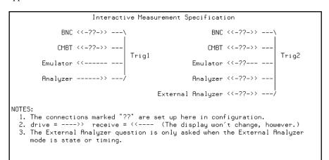
This display illustrates the possible connections between the internal lines (trig1 and trig2) and the emulator, analyzer, and external devices.
