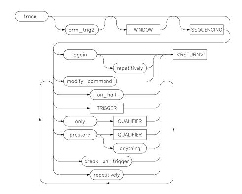
This command allows you to trace program execution using the emulation analyzer.
