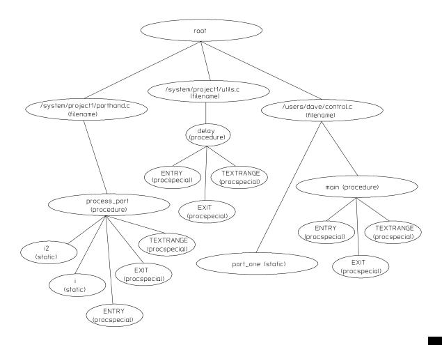
SRU does not build tree nodes for variables that are dynamically allocated on the stack at run-time, such as i and j within the delay() procedure. SRU has no way of knowing where these variables will be at run time and therefore cannot build a corresponding symbol tree entry with run-time addresses.
