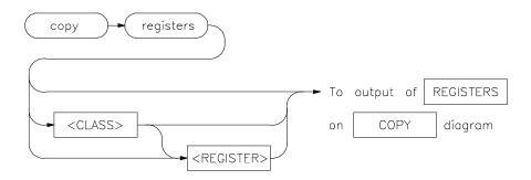
This command copies the contents of the processor registers to a file or printer.
