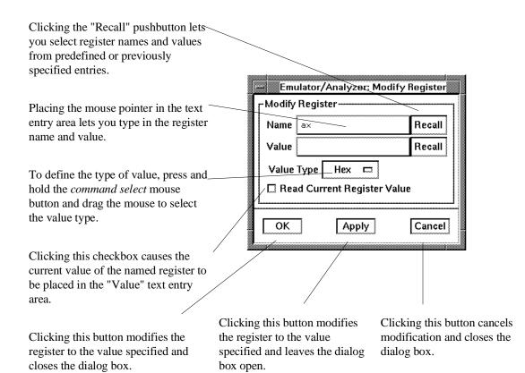
• Using the command line, enter the **modify register < register> to < value>** command.
