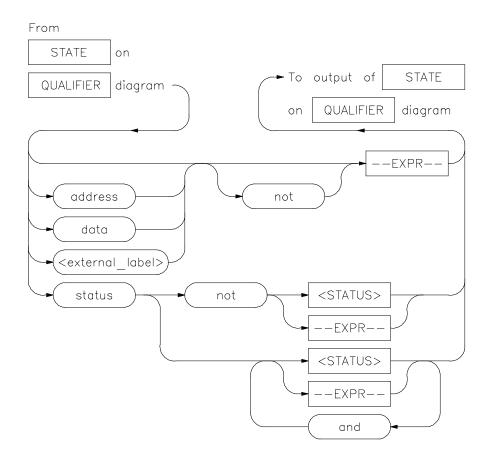
This parameter lets you specify a trigger condition as a unique combination of address, data, status, and executed address values.
