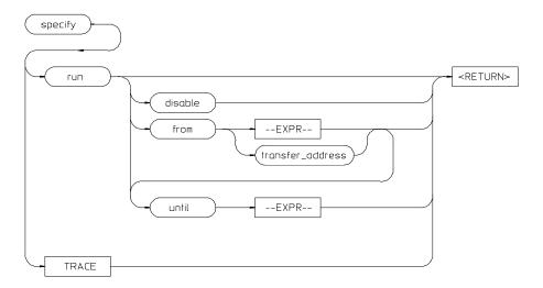
This command prepares a **run** or **trace** command for execution, and is used with the **cmb\_execute** command.
