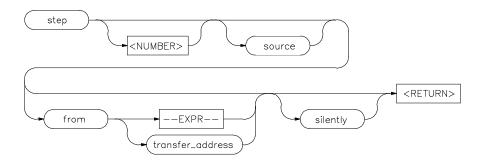
The **step** command allows sequential analysis of program instructions by causing the emulation processor to execute a specified number of assembly instructions or source lines.
