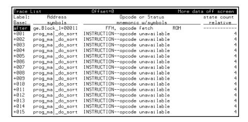
The trace listing above shows that the program loops 4 times for each call of the "do sort" function.
