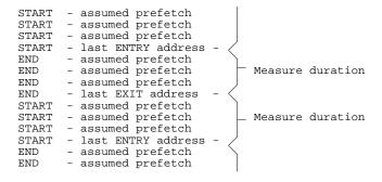
When measuring a recursive function, module duration will be measured between the last recursive call and the true end of the recursive execution. This will affect the accuracy of the measurement.
