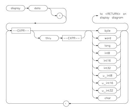
The **display data** command can display the values of simple data types in your program. Using this command can save you time; otherwise, you would need to search through memory displays for the location and value of a particular variable.
