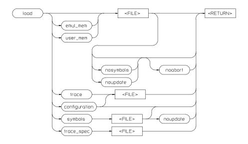
This command transfers absolute files from the host computer into emulation or target system RAM. With other parameters, the load command can load emulator configuration files, trace records, trace specifications, or symbol files.
