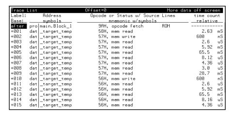
Notice the trigger state (line 0, labeled "after") is included in the trace list; trigger states are always stored.
