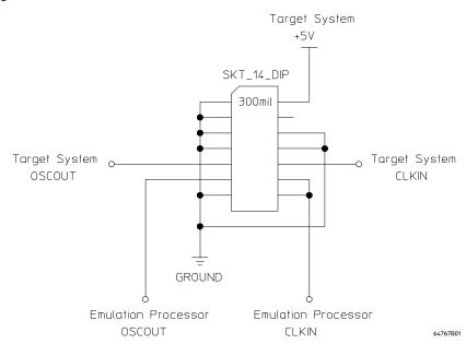
A jumper that connects the emulation processor OSCOUT and CLKIN pins to the OSCOUT and CLKIN pins on the target connector is provided. You can use this jumper if:
