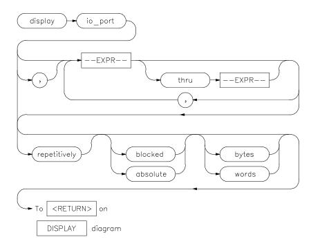
This command displays the contents of the specified I/O port location or series of locations.
