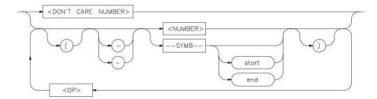
An expression is a combination of numeric values, symbols, operators, and parentheses used to specify address, data, status, executed address, or any other value used in the emulation commands.
