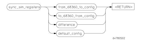
The **sync\_sim\_registers** command synchronizes the 68360's system integration module (SIM) registers to the emulator's EMSIM registers.
