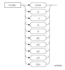
The function code is used to define the address space being referenced. Select the appropriate function code from those listed below.
