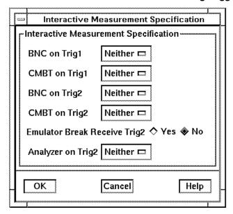
If you're using the Softkey Interface from a terminal or terminal emulation window, you don't get a dialog box from which to choose configuration sections; however, you have access to the same configuration options through a series of configuration questions. To access the questions in the "Interactive Measurement Specification" section, answer "yes" to the "Modify interactive measurement specification?" question.
