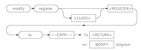
This command allows you to modify the contents of the emulation processor internal registers.
