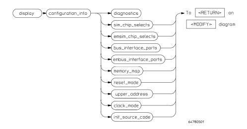
The **display configuration\_info** command displays information about emulator configuration and processor SIM programming. You can also display diagnostic information about inconsistencies found in the emulator configuration.
