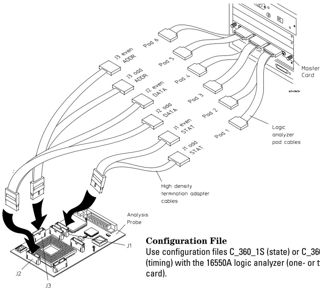
Expansion card connections for a two-card Agilent Technologies 16550A logic analyzer. Connection of J4, J5, and J6 is optional.
