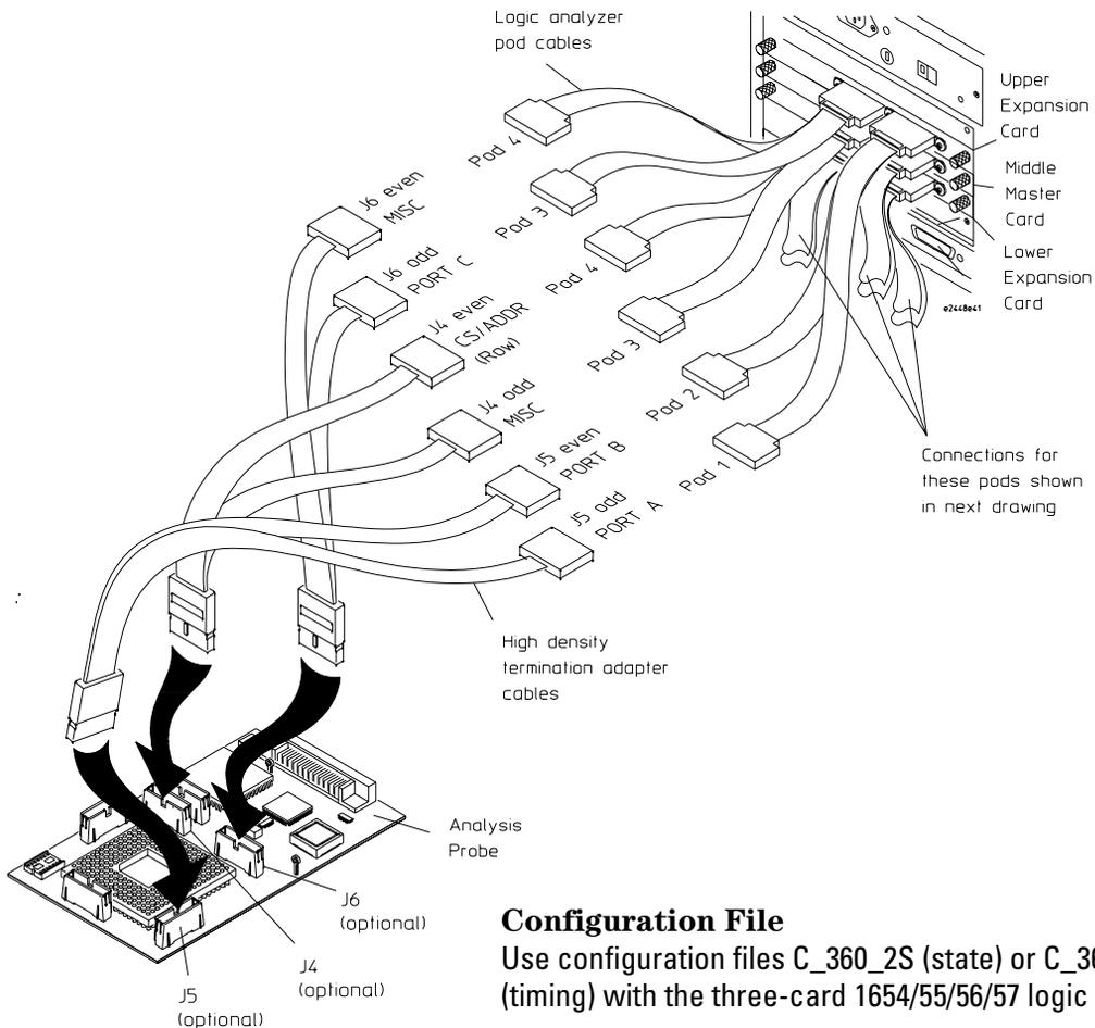
Three-card Agilent Technologies 16554/55/56/57 logic analyzer connections (continued)
