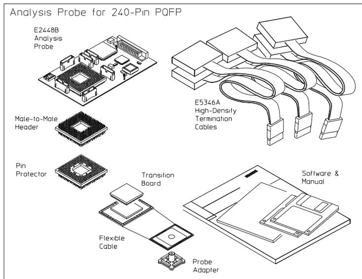
**Equipment Supplied with the Agilent Technologies E2448B Analysis Probe**
