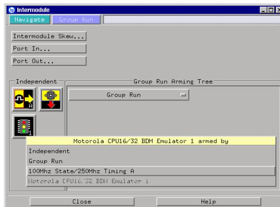
The emulation module is now set to stop the processor when the logic analyzer triggers.
