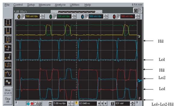
Fig 9b : Analog channel Add Agilent E4838A Frontend
