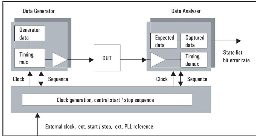
Figure 2: Block Diagram of 81200 functional layout
