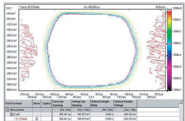
Figure 13a) b): Signal of E4861A with E4862A and E4863A Analyzer
