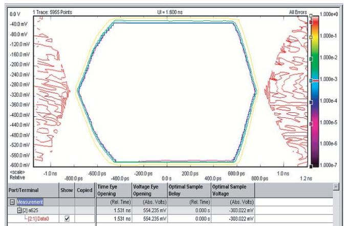
Figure 12 a) b): Signals of E4832A with E4838A Generator + E4835A Analyzer
