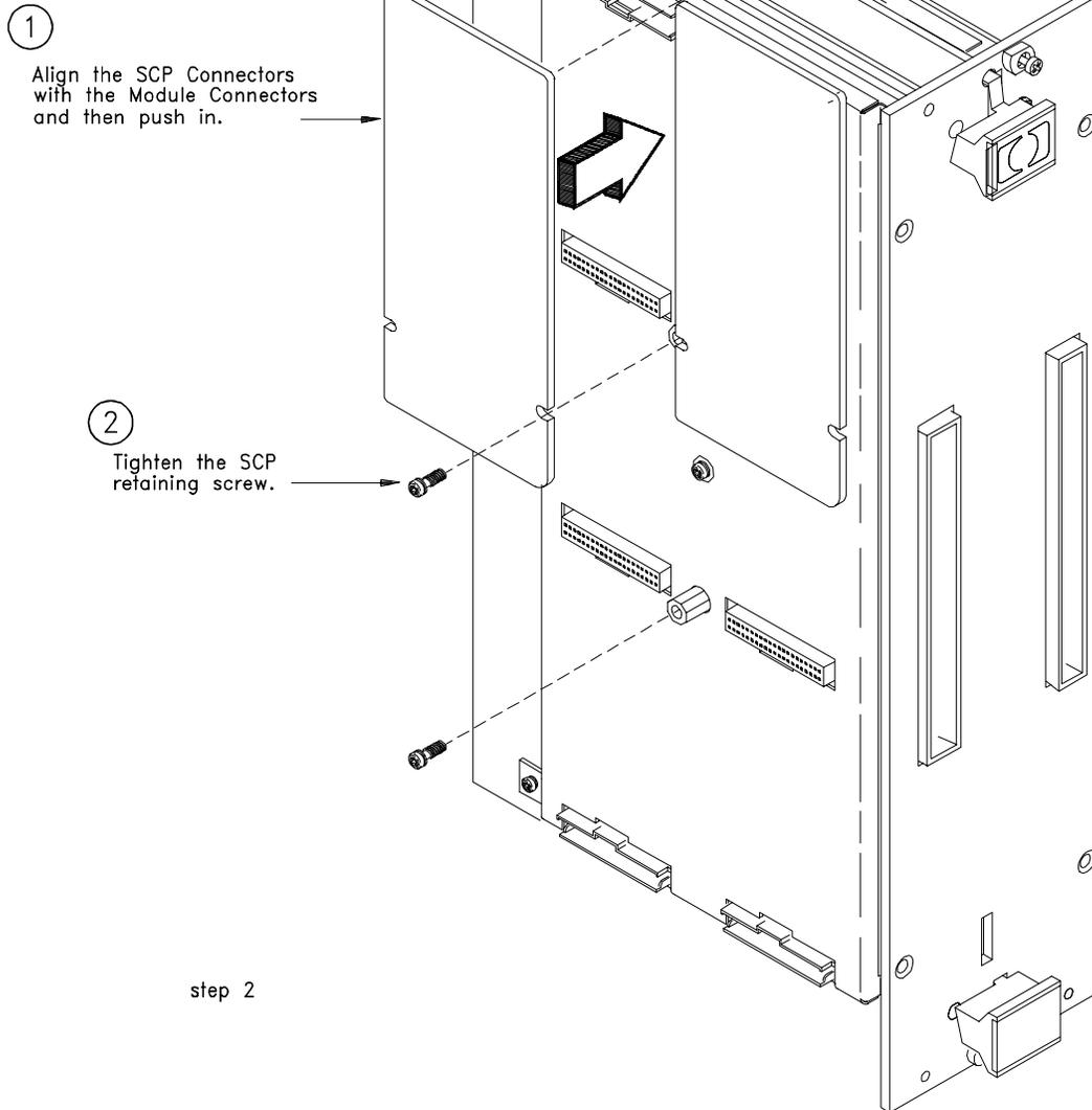
**NOTE:** No more than four HP E1510A Sample and Hold (Option 020) SCPs can be used with an individual HP E1313A.
