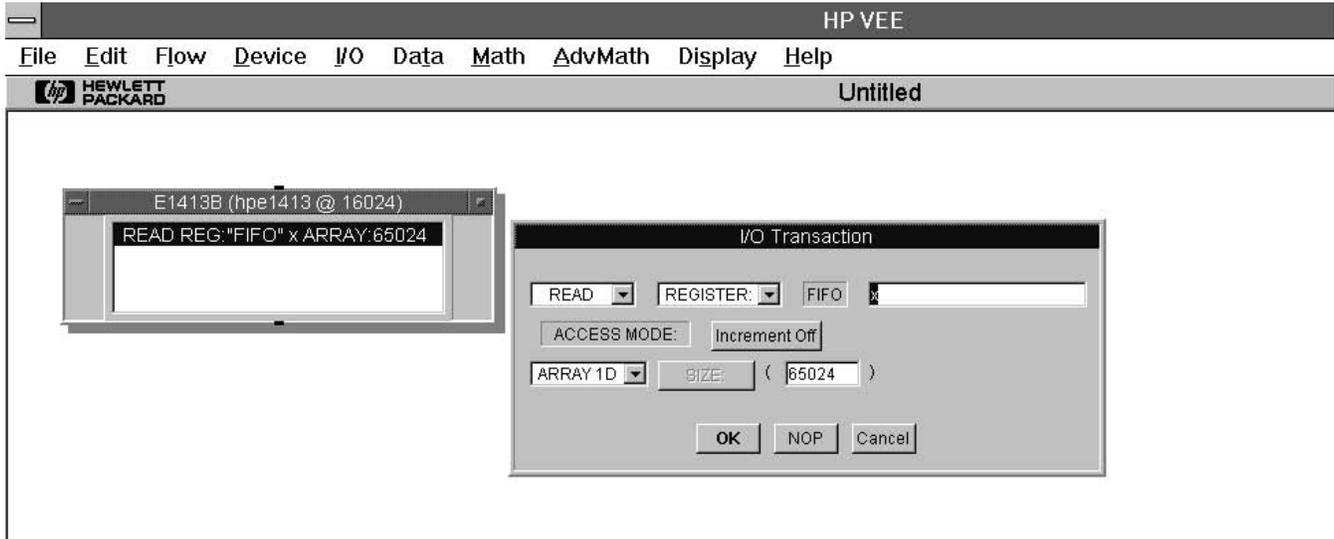
This sets HP VEE up to read the register that in step 2 we named “FIFO” and store the results in variable X.
