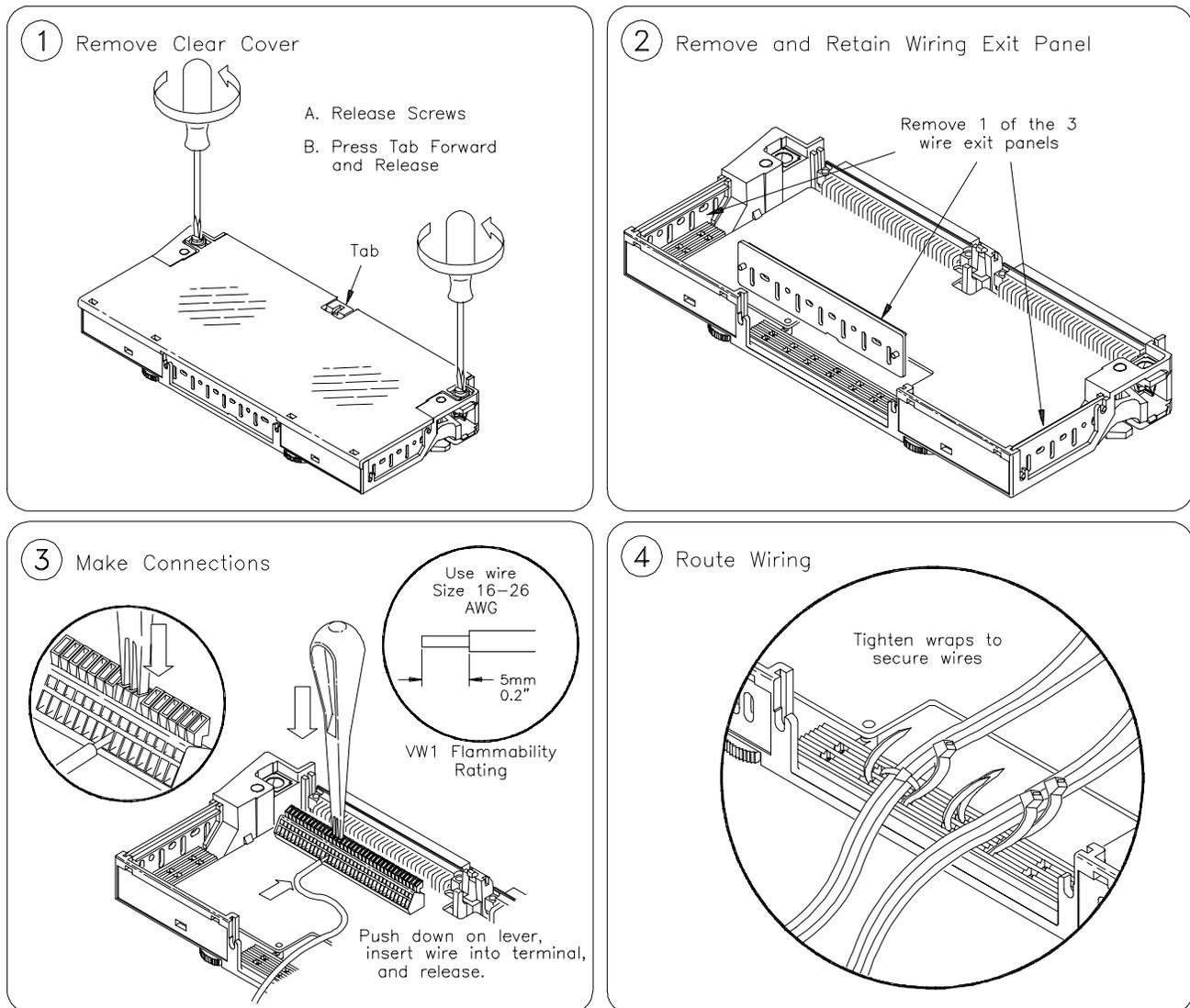
Figure 2-16. Wiring the HP E1413 Terminal Module
