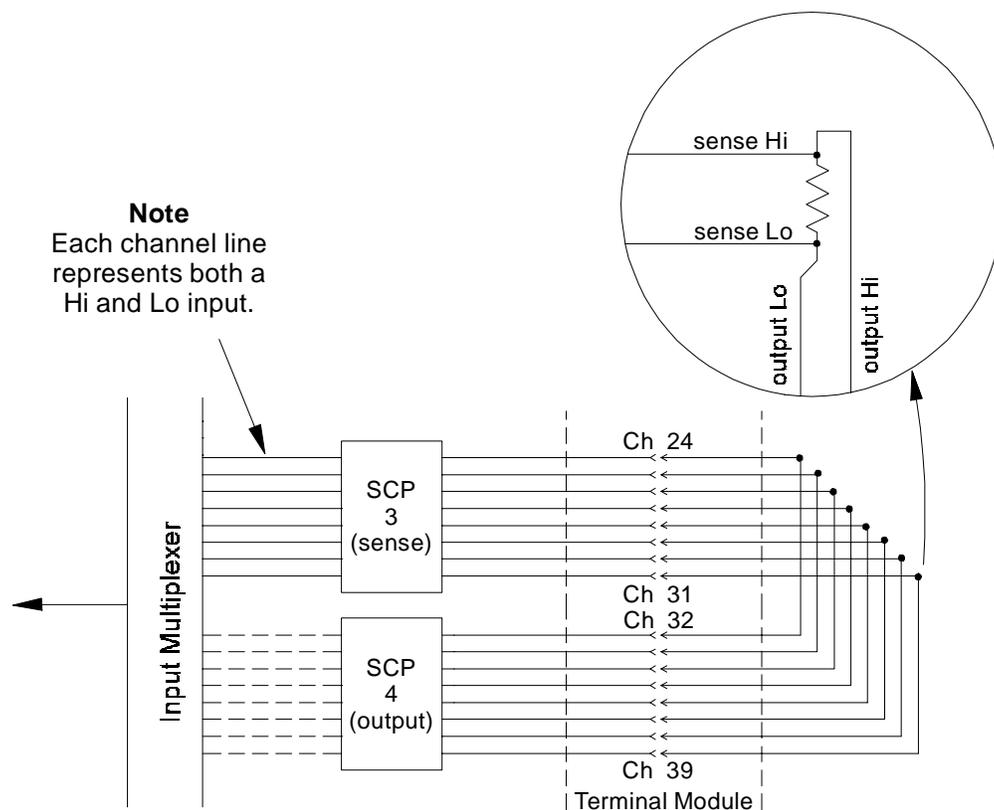
Figure 2-2. Pairing Output and Sense SCP Channels
