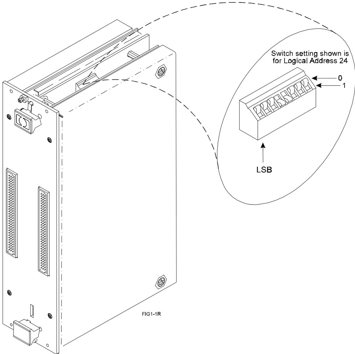
Figure 1-1. Setting the HP E1313 Logical Address
