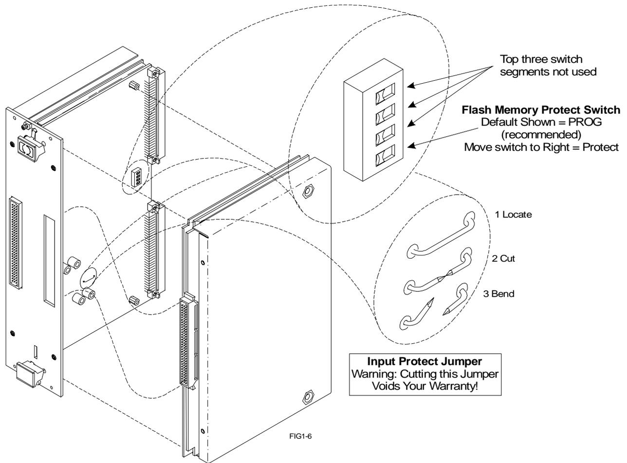
Figure 1-3. Locate and Access JM2201 and JM2202 on HP E1313
