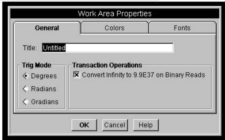
This sets up HP VEE so it can directly access data from the HP E1313/E1413 FIFO and CVT registers. This is required because the HP E1313/E1413 has implemented IEEE 754 Floating Point Format which includes special codes for “plus infinity”, “minus infinity”, and “not a number”. These special codes causes a floating point math error in HP VEE, thus they must be converted to a number which HP VEE can handle such as 9.9E37.
