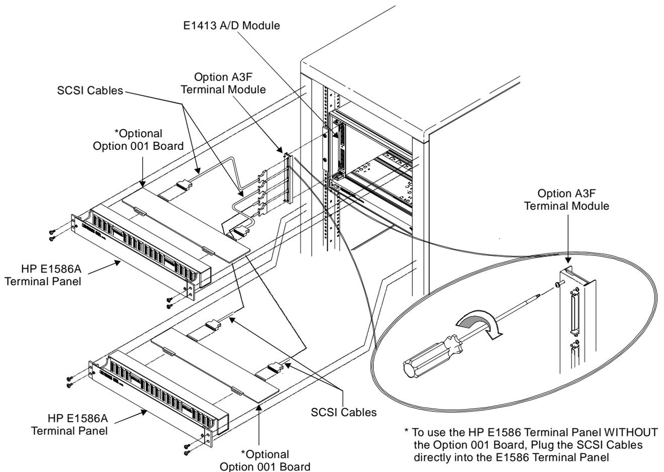
Figure 2-25. Connecting the HP E1586A Rack Mount Terminal Panel
