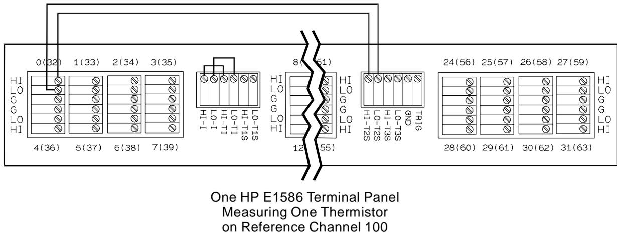
**Figure 3-8. Center Thermistor Measurements on a Single Panel**
