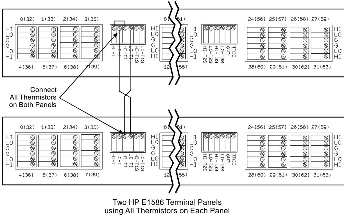
**Figure 3-7. Connecting Six Thermistors on Two Panels**
