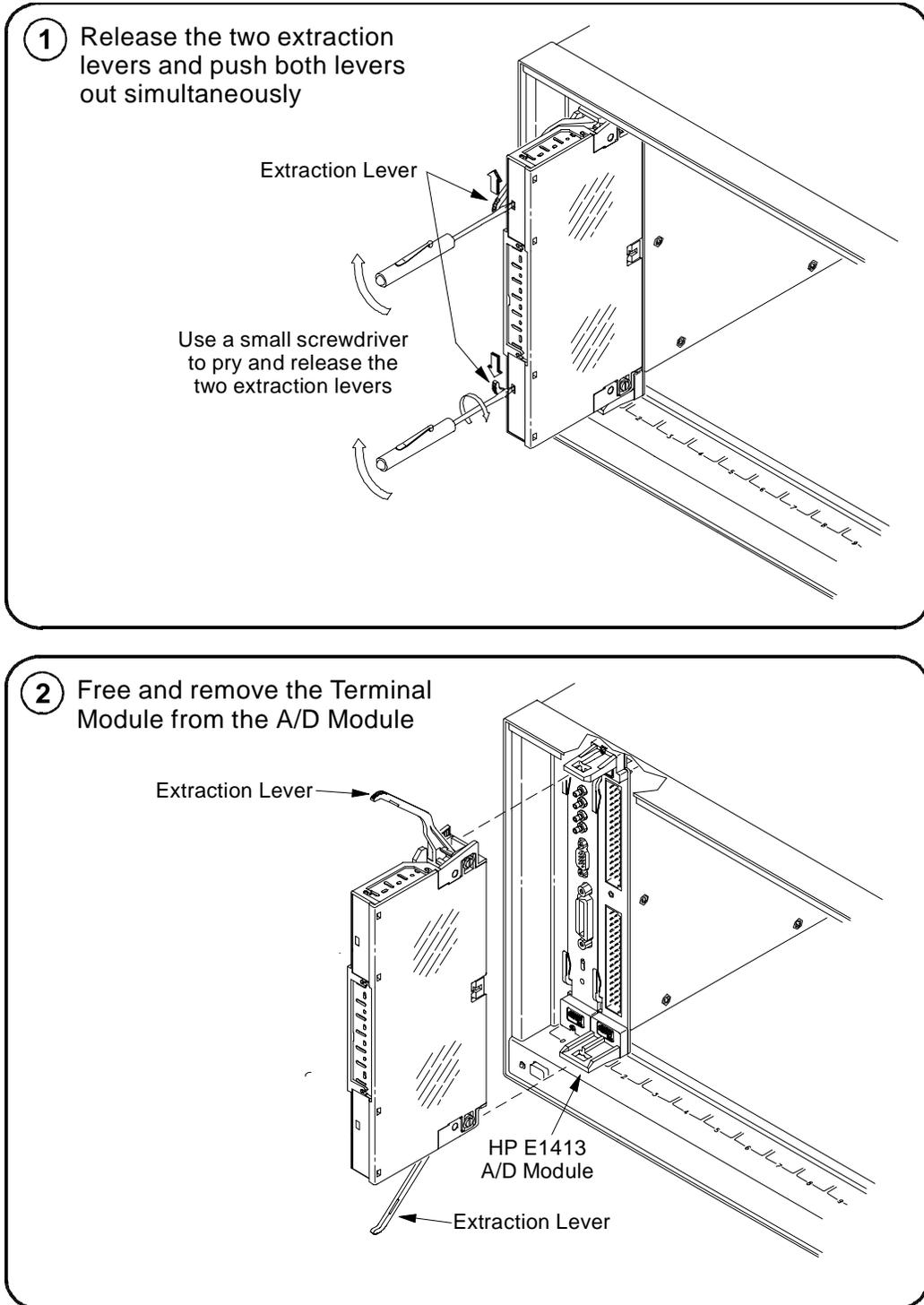
Figure 2-18. Removing the HP E1413 Terminal Module
