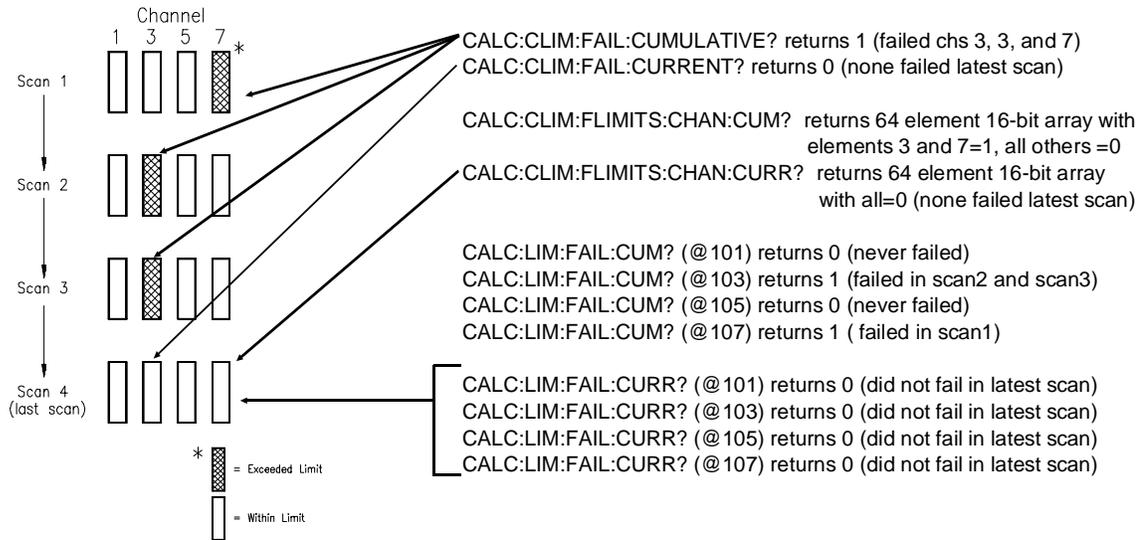
Figure 4-8. Querying Limit Test Results
