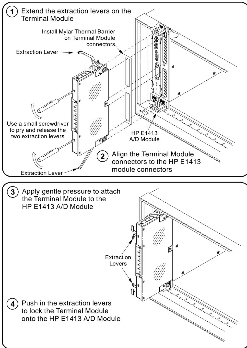
Figure 2-17. Attaching the HP E1413 Terminal Module
