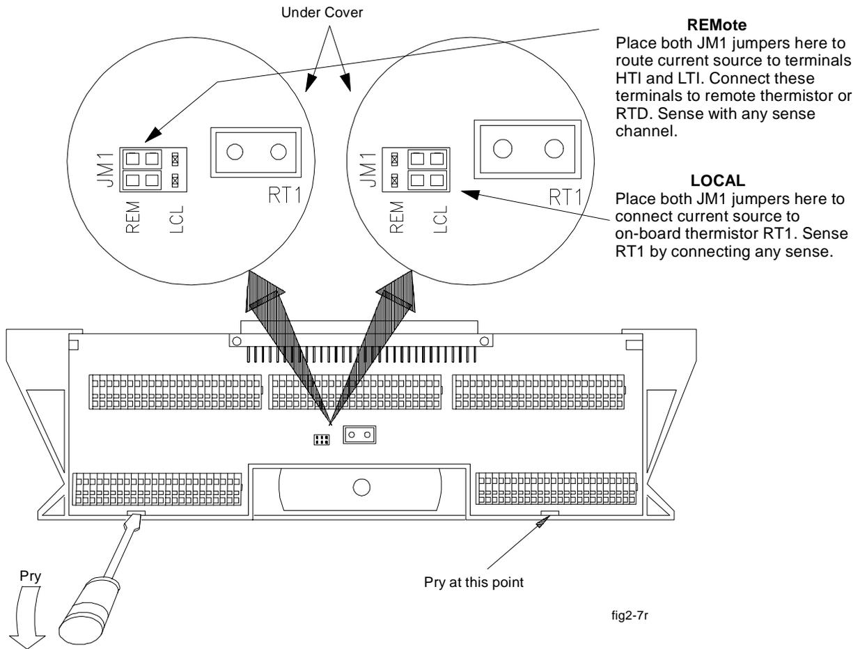
**Figure 2-11. Temperature Sensing for HP E1313 Terminal Module**
