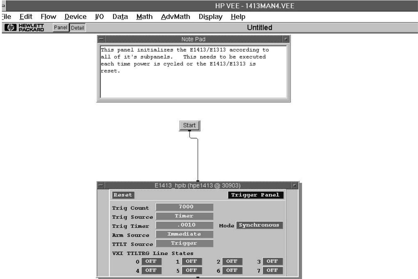
This part of the program starts the measurement and then transfers the readings to the computer. The READ BINARY x BYTE ARRAY:9 reads the IEEE 488.2 arbitrary block header. The block header has the form of #nnd where:
