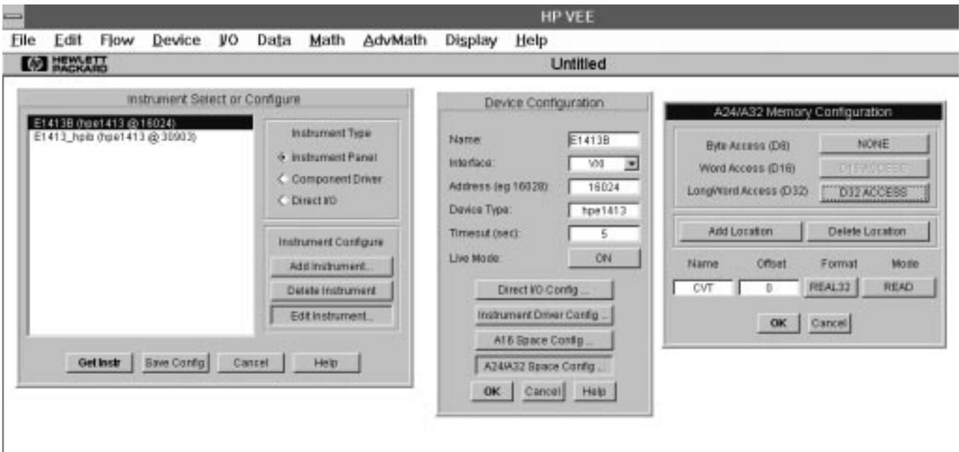
The HP E1313/E1413 current value table is located in A24 address space. Each channel is a 32-bit real number with Channel 0 at offset 0, channel 1 is at offset 4, and so on.
