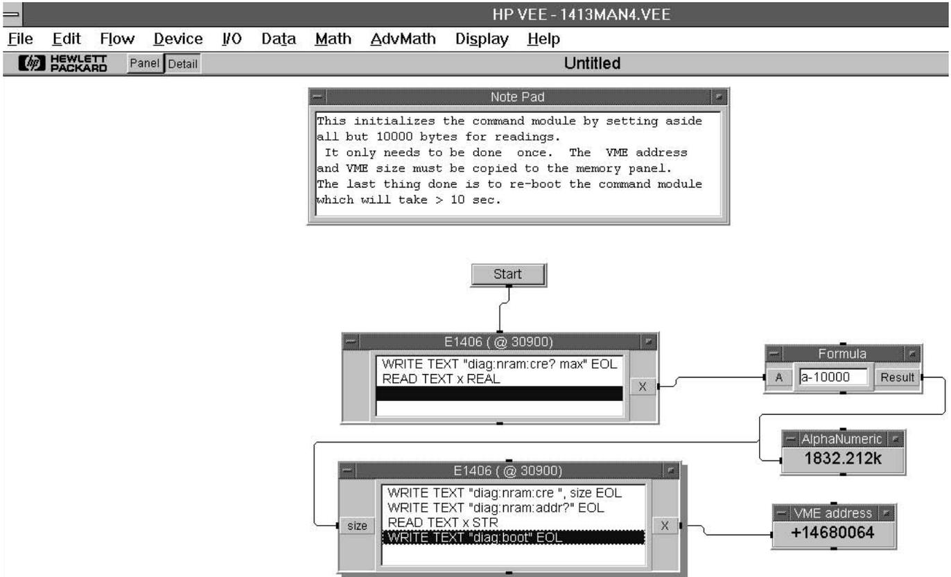
Once the command module has been configured, then use an HP E1413 instrument panel to configure the HP E1313/E1413.
