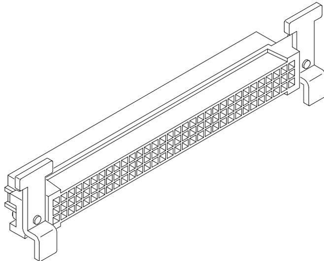
**Figure 2-21. Crimp-and-Insert Connector**
