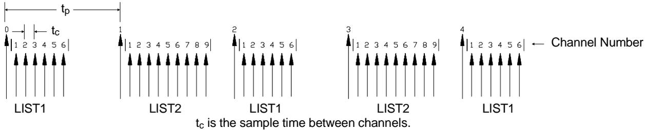
The large arrow is the pacing Trigger Timer. The smaller arrows are sample triggers generated by the HP E1313/E1413 when stepping through the channel list. The first large arrow is the arming event.
