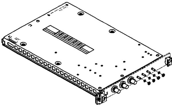
2 Using a 9/16-inch open-end wrench, remove the washers and nuts from the BNC connectors.
