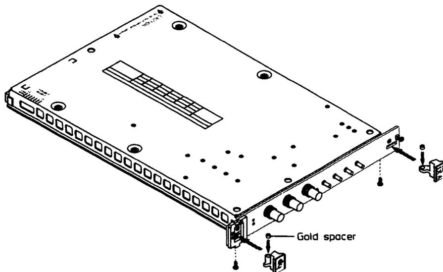
4 Using a T-10 torx driver, remove the screw that attaches the front panel to the main assembly.
