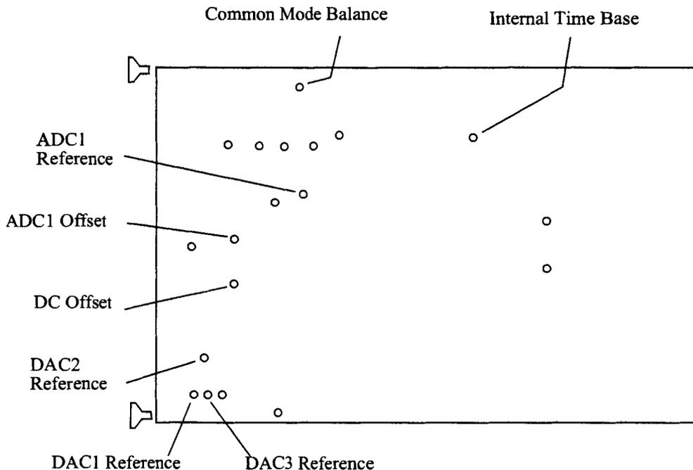
**Set up for adjusting and measuring common mode characteristics**
