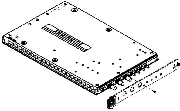
5 To replace the front panel with another that does not have its own side brackets, remove the brackets from the old front panel. Use a T-8 torx driver.
