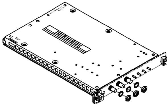
3 Using a T-8 torx driver, remove the screws that attach the handles. The screws come out from below. The screws pass through a gold spacer; be careful not to lose the spacer when the handle is removed.
