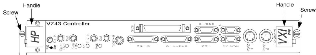
**Figure A-1. Extracting the Controller**
