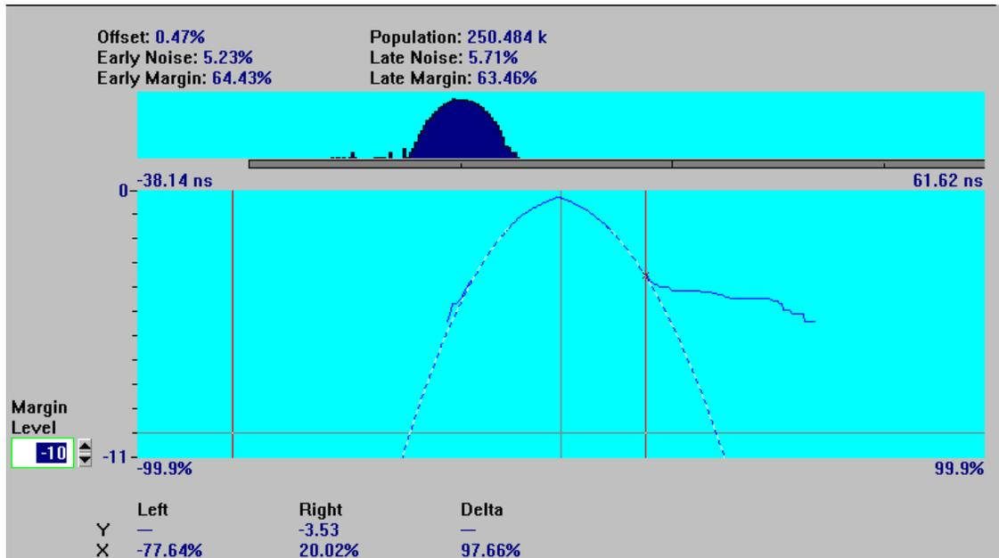
Notice that the new late window curve fit ignores the break-away in the window margin data and more closely approximates the rest of the acquired data in the window margin curve. The resulting margin is much closer to the early window margin.
