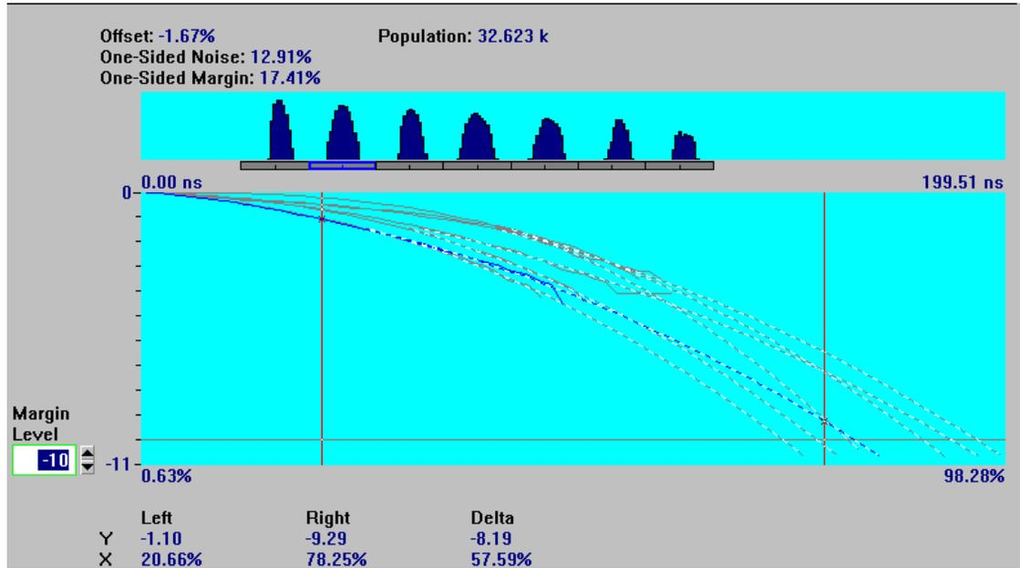
This display shows the one-sided window margin plot, with the segments overlaid. The one-side margin plot is computed by “folding” all of the distributions about the segment centers, adding the selected segments together, and computing window margin from this single-sided histogram.
