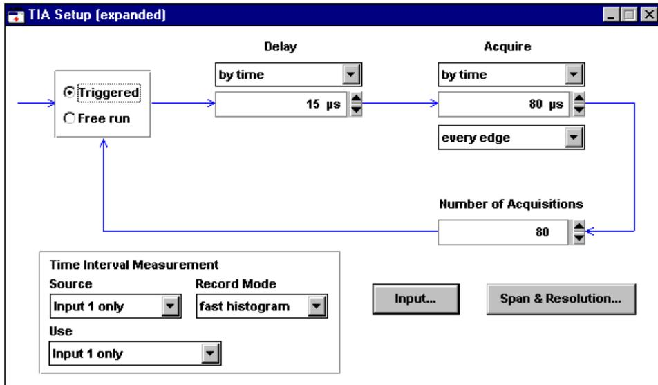
This is the TIA setup menu to make data-to-data measurements on the drive under test. The screen is configured as a flow diagram showing the various stages of the measurement. Reading from left-to-right you can see that the TIA will wait for a trigger, delay 15  $\mu\text{s}$  and then measure every edge for 80  $\mu\text{s}$ . This sequence is repeated 80 times, which results in the acquisition of 80 consecutive sectors.
