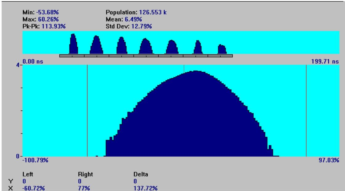
This result display allows you to analyze histograms by defined “segments” or decode windows. The panorama display shows the individual distributions as with the previous histogram display, but the main display shows the histograms combined, or added together based upon the segment definition. Notice the darkened grid beneath the panorama display. This represents the currently defined segments. The half tic mark represents the center of each segment.
