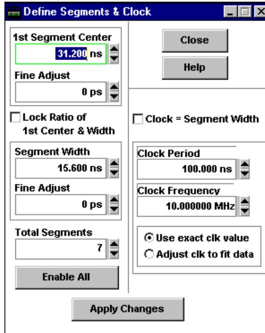
This window allows you to define the number and position of the segments and define the clock. Since this drive has a 15.6 ns decode window, the first distribution (2T) is located at 31.2 ns. The RLL (1,7) coding dictates that there should be 7 segments. These segment definitions are also used for window margin calculations. Since data-to-data intervals are used for display and analysis for this demonstration (instead of data-to-clock), the clock definition is not required.
