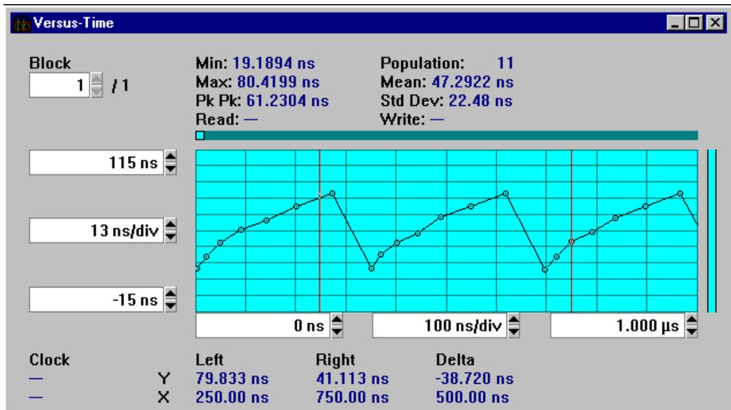
You can see the time order of the measured time intervals. There is a repeating pattern of seven time intervals. Each one corresponds to a distribution you saw earlier in the histogram data. The y-axis shows the time interval values, between 19 and 80 ns. The x-axis shows the time-of-occurrence for each measured interval.
