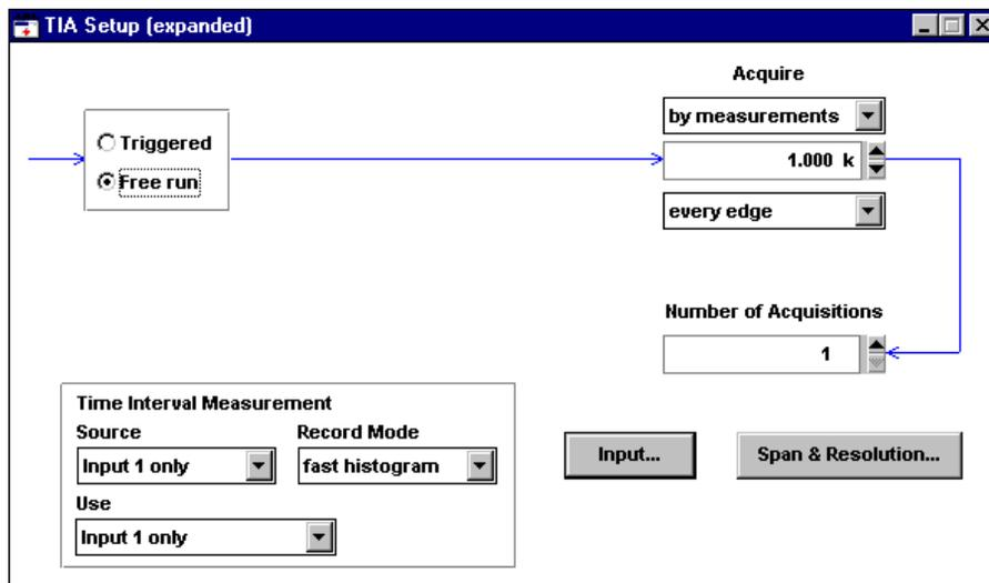
This window is used to specify how the TIA will acquire measurement data. As specified on this setup form, you will make a fast histogram acquisition consisting of 1,000 measurements. They will be single-source measurements as would be used when making data-to-data measurements and these measurements will be used for display and analysis.
