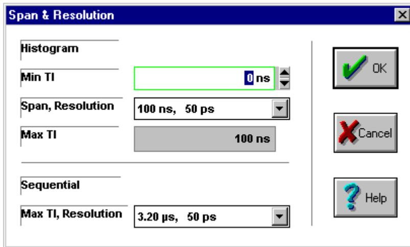
A dialog box is opened. There are two parts to this form, Histogram and Sequential. The upper part sets the boundaries for the histogram, the lower sets the boundaries for sequential measurements.
