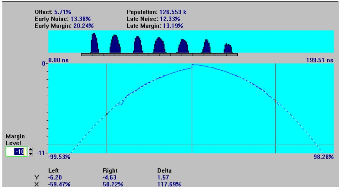
This display shows window margin computed from the histogram, using the segment definitions created earlier. The panorama display shows the original histogram distributions, and the main display shows the computed two-sided window margin. The dashed line is the extrapolated curve through  $10^{-10}$  margin level.
