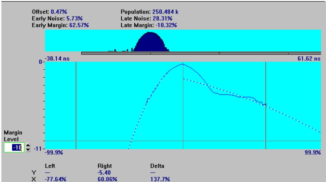
These are the corresponding window margin results for the data-to-clock histogram. Due to the incorrect delay from trigger value, the histogram (shown above the window margin) has a number of measured intervals that are set apart from the main distribution. You can see these on the left side of the histogram on the panorama display.
