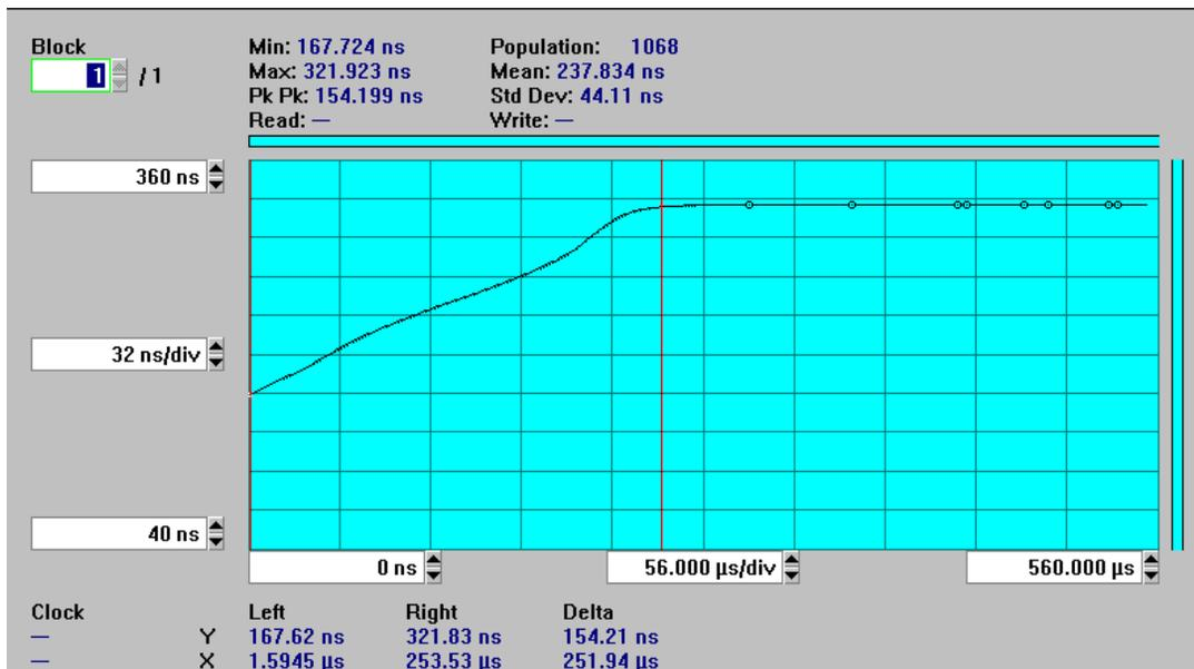
This is the HP E1741A's "measurement" vs. time display of sequential, or continuous, measurement data. In this example, the display is "time interval vs. time." The markers work much the same as for the histogram display, as you can click on either one with the mouse and drag it to the desired location. Statistical values are presented at the top of the display for the data between the current position of the markers. Marker values and differences are displayed at the bottom of the display.
