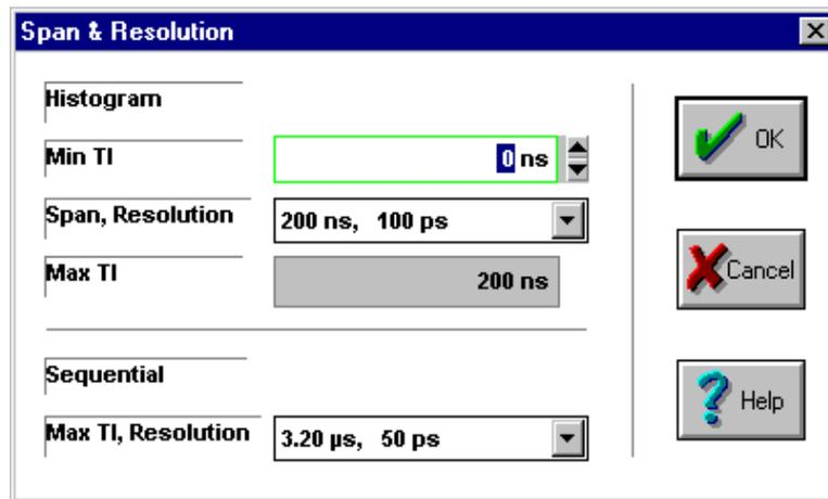
This window configures the fast histogram hardware to cover the range of intervals being measured. Since this drive has a decode window or “T” spacing of 15.6 ns and uses RLL (1,7) coding, intervals will cover the range from 2T to 8T (31.2 ns nominal to 124.8 ns nominal). A span of 200 ns is chosen to cover this measurement range for the histogram. The resulting histogram bin width, or resolution, is 100 ps.
