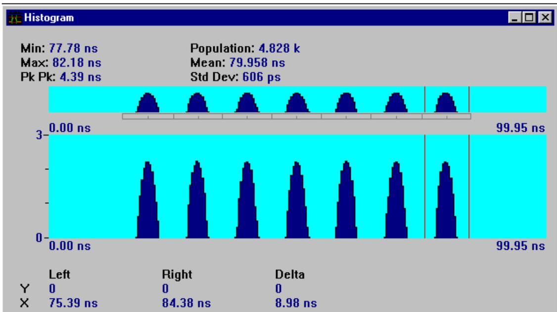
Now you can read the statistics for one distribution. The panorama display (the display just below the statistics) always shows the entire span of the histogram, while the main display below can be scaled to show a closer view of the data.
