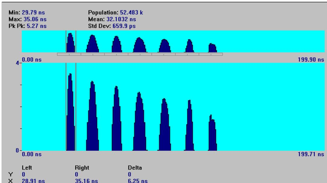
This histogram result display clearly shows the seven time interval distributions corresponding to the 2T through 8T code spacings. The upper display is called the panorama display and always shows a full view of all the data acquired. You can “zoom-in” or magnify the data by pressing the **↑** key on the keyboard. The larger, main display will show the magnified view.
