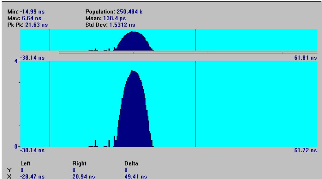
This histogram display shows a single histogram distribution, corresponding to the data-to-clock measurement configuration. With dual-channel measurements there are often systematic timing differences (skew) between the measured edges of each channel. This can occur for numerous reasons: cable length differences, propagation delays in circuit access points, etc. The TIA has been calibrated so that internal path length differences should not contribute significant timing skew.
