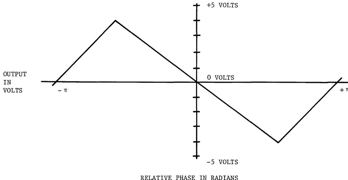
**FIGURE 4-12 COARSE DATA PHASE DETECTOR CHARACTERISTIC**
