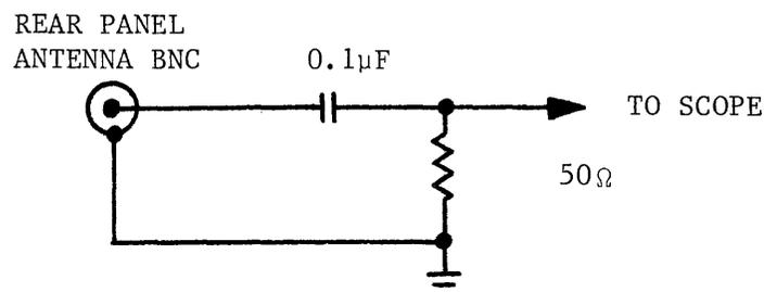
FIGURE 5-3      50 OHM DUMMY LOAD
