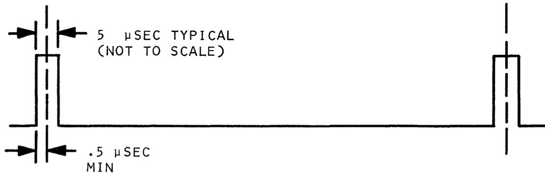
FIGURE 3-5 MILLISECOND COUNTER TIMING DIAGRAM 1 kHz SIGNAL SHOWN
