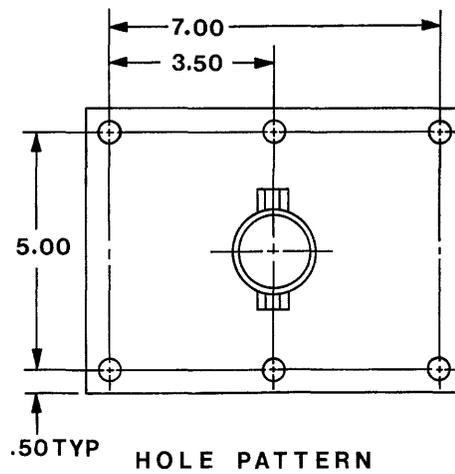
FIGURE 7-2 BASE, ANTENNA MOUNTING DIMENSIONS
