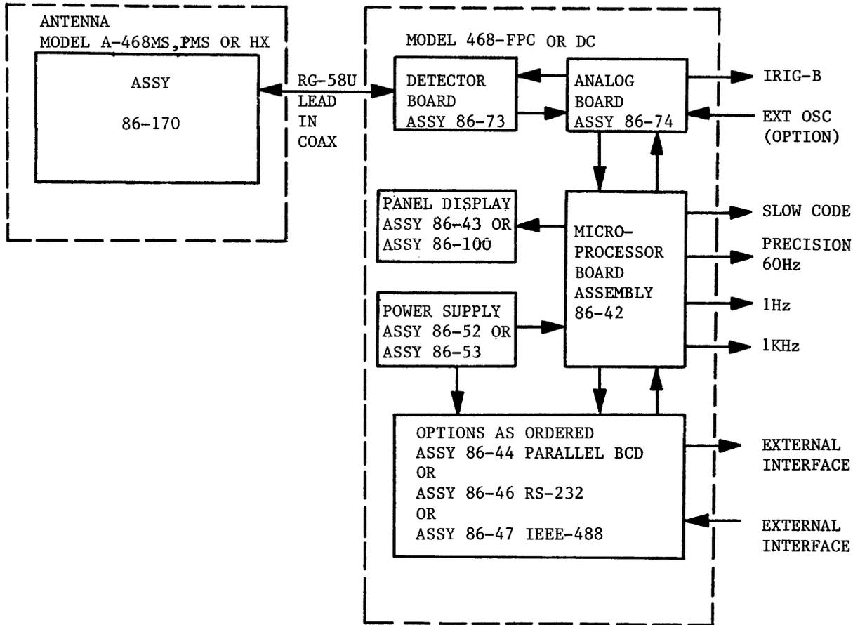
FIGURE 4-2 OVERALL BLOCK DIAGRAM - MODEL 468-DC
