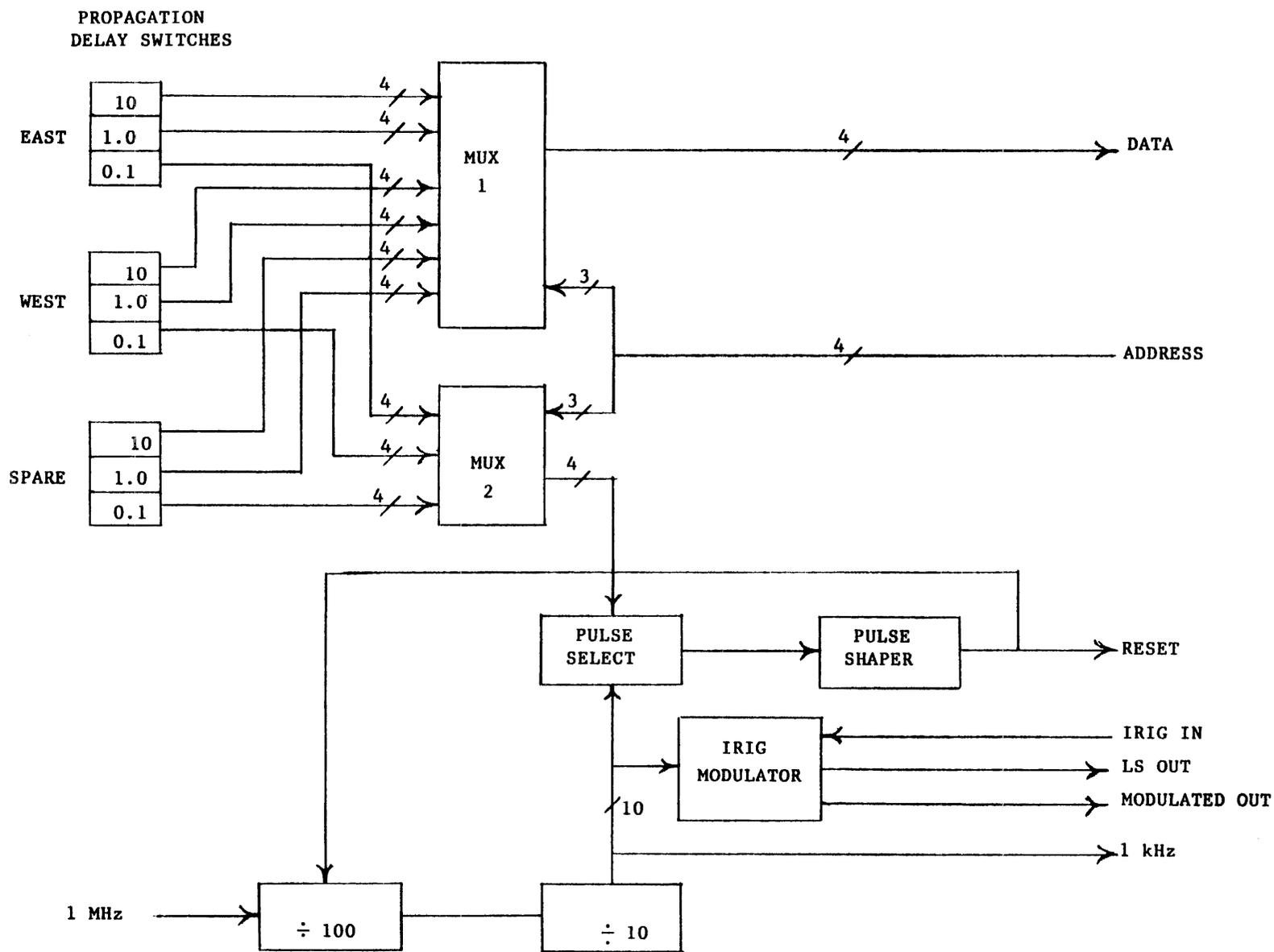
'EAST', 'WEST', and 'SPARE', respectively. Each switch is labeled '10', '1.0', or '0.1', indicating the multiplier value of the switch setting in milliseconds.
