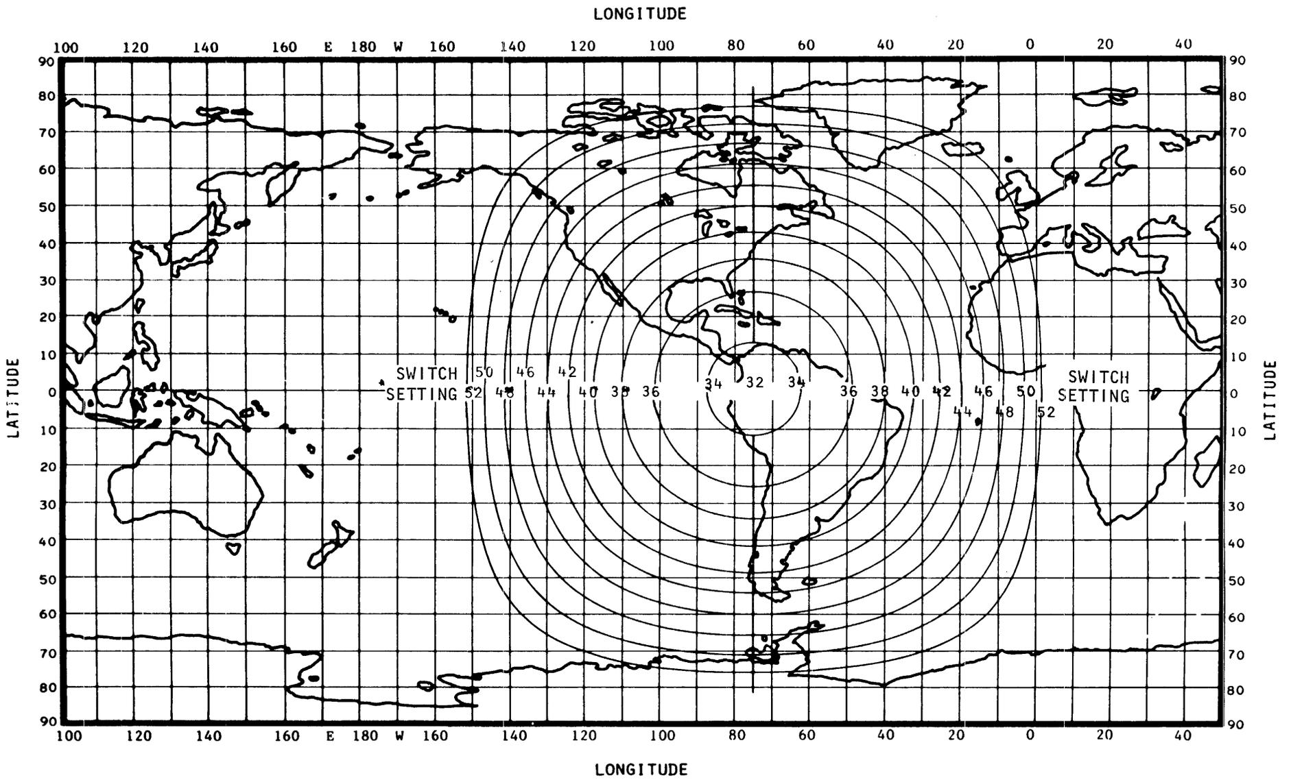
FIGURE 3-2 EASTERN SATELLITE MEAN DELAYS
