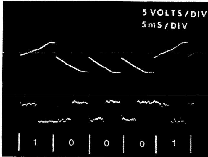
FIGURE 4-8 DATA INTEGRATOR OUTPUT
