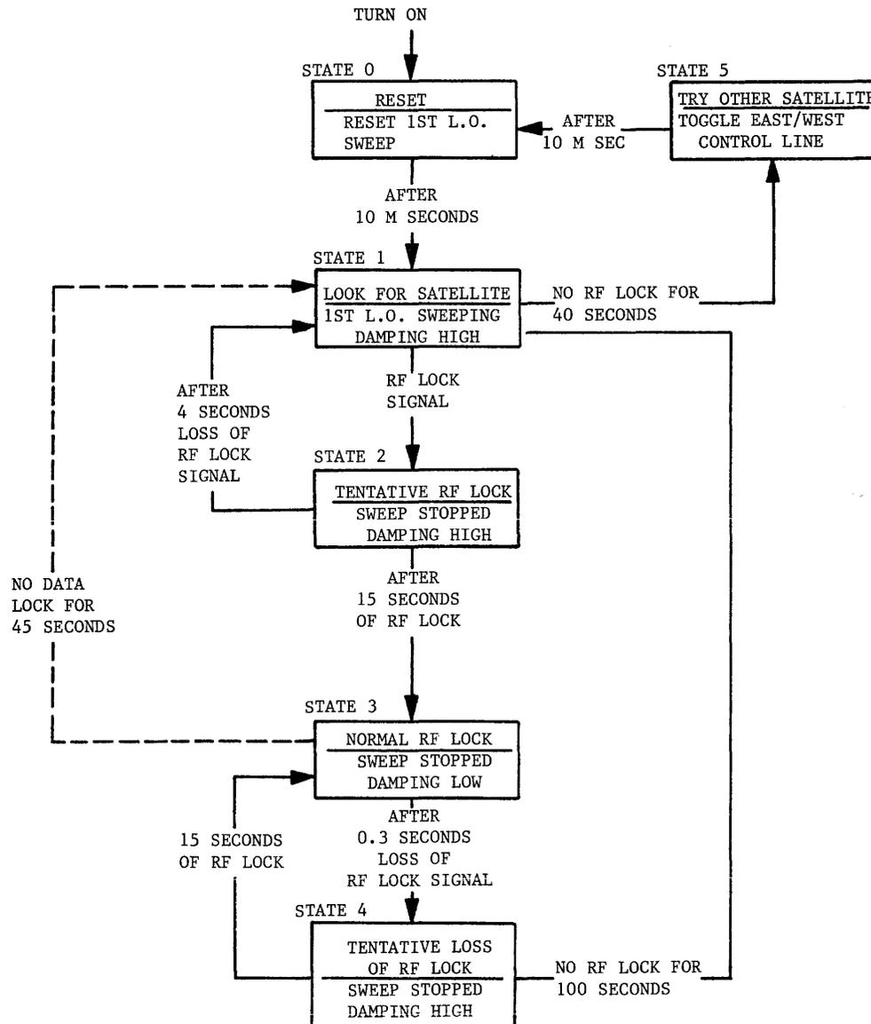
FIGURE 4-17 RF LOCK STATE DIAGRAM
