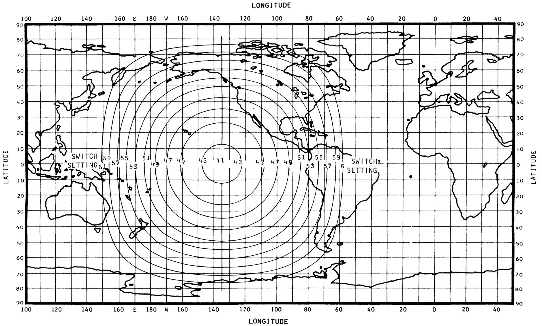
FIGURE 3-1 WESTERN SATELLITE MEAN DELAYS
