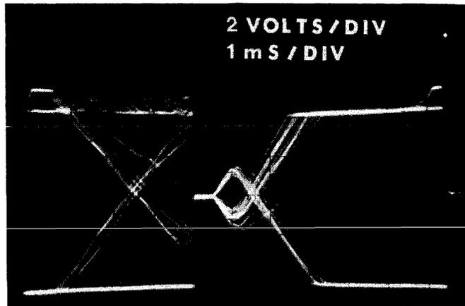
FIGURE 4-13 FINE DATA PHASE DETECTOR INTEGRATOR OUTPUT
