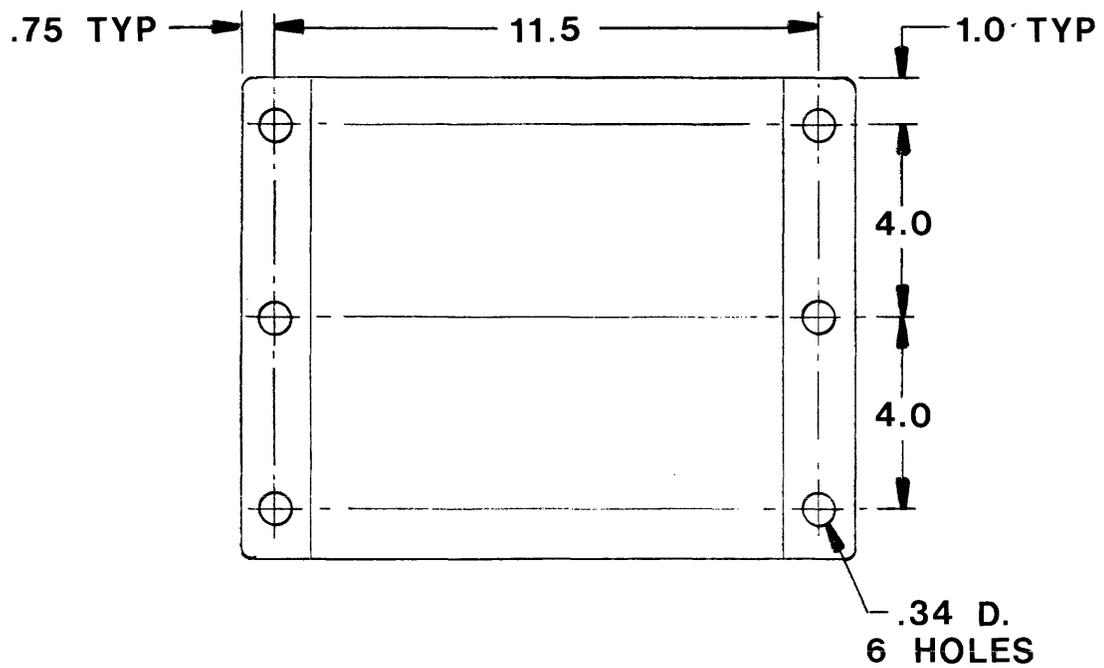
FIGURE 7-5 A-468RK AND A-468RKC MOUNTING DIMENSIONS
