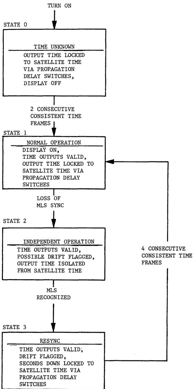
**FIGURE 4-19 FRAME SYNC CONTROL STATE DIAGRAM**
