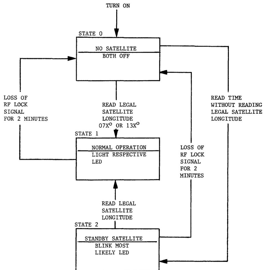
FIGURE 4-21 SATELLITE LED STATE DIAGRAM
