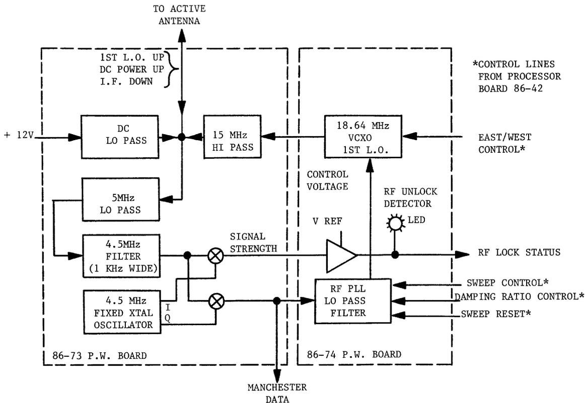
**FIGURE 4-4 PHASE LOCK LOOP BLOCK DIAGRAM - MODEL 468-DC**
