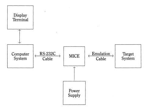
When a computer system is interfaced to the MICE module, a driver program must be resident in the computer system. Driver programs for various systems have already been written, including
