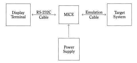
If a computer system is used as the controlling device, the configuration is similar to the one above; the computer with its display terminal now replaces the lone terminal.
