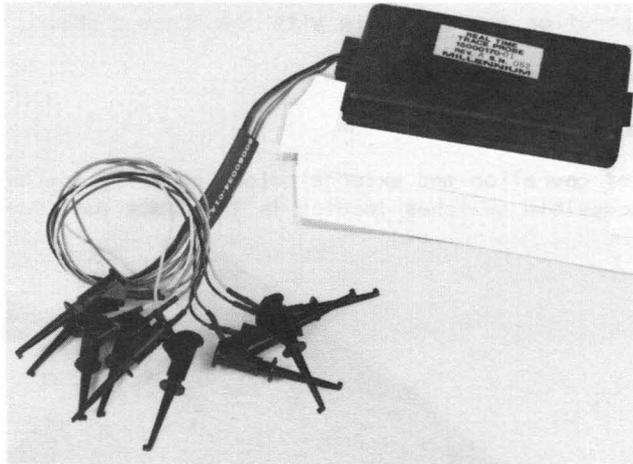
Figure 5-1. External Test Clips Probe
