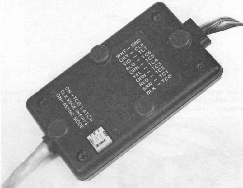
Figure 5-3. Operation and Clock Polarity Switches
