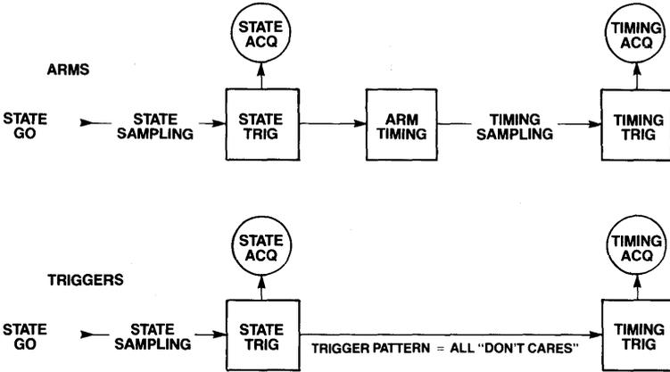
Figure 6-7. State Arms/Triggers Timing.
