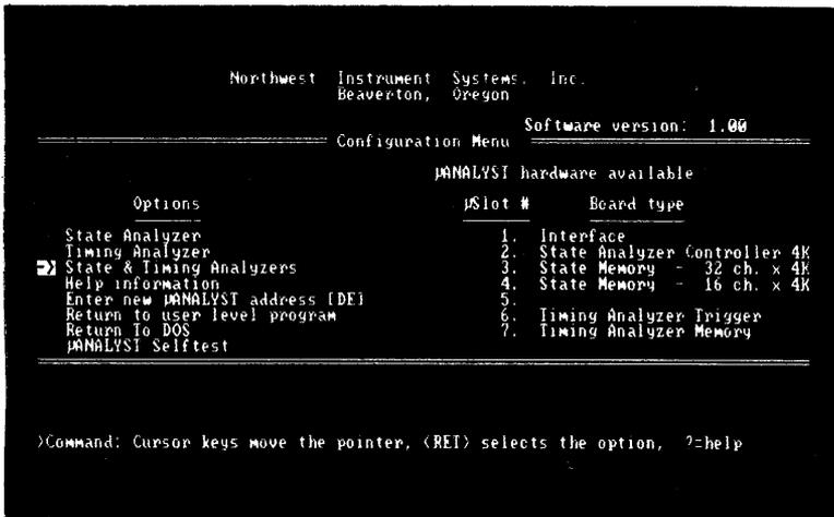
■ Figure 6-1. The Configuration Menu when the state and timing analyzers are both installed in the  $\mu$ Analyst mainframe.
