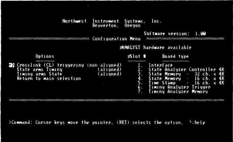
■ Figure 6-2. Aligned/non-aligned acquisition modes.
