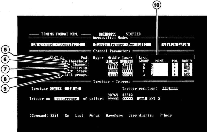
■ Figure 5-6. The Format Menu and its fields for controlling channel parameters.
