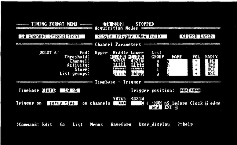
■ Figure 5-9: Setup and Hold Time fields in the Format Menu.
