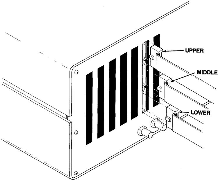
■ **Figure 2-13. Connecting the probes to the trigger board.**
