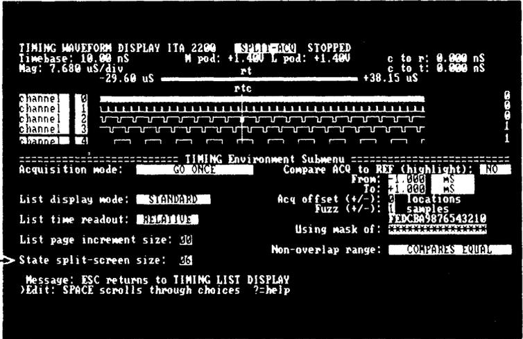
**Figure 6-6. Selecting the size of the split-screen display in the timing analyzer's Environment Submenu.**
