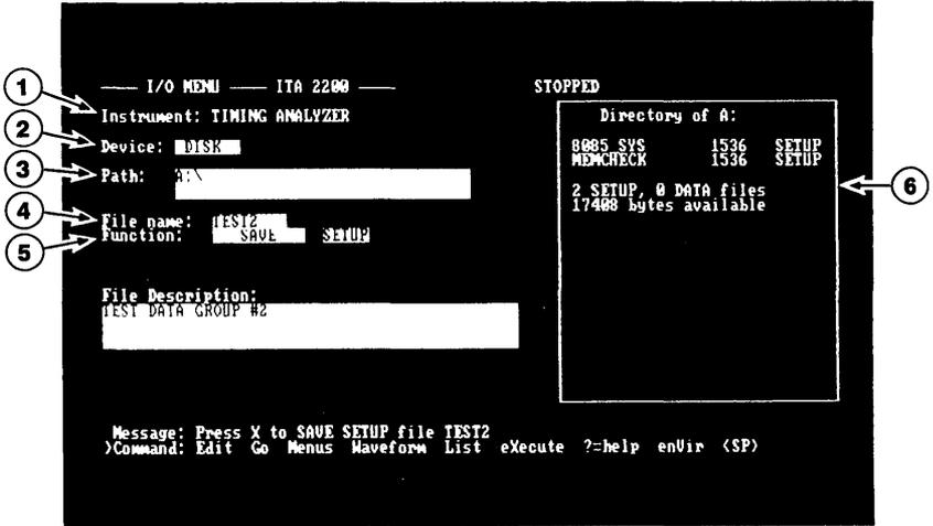
■ Figure 5-24. The I/O Menu with DISK as the selected device.
