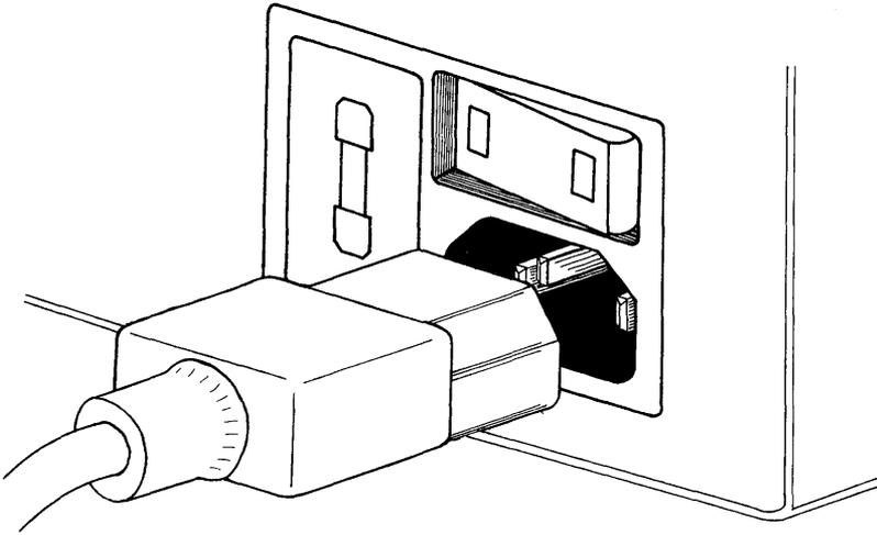
■ **Figure 2-5. Connecting the power cord.**
