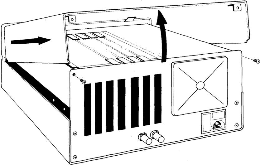
■ **Figure 2-9. Removing the mainframe's cover.**
