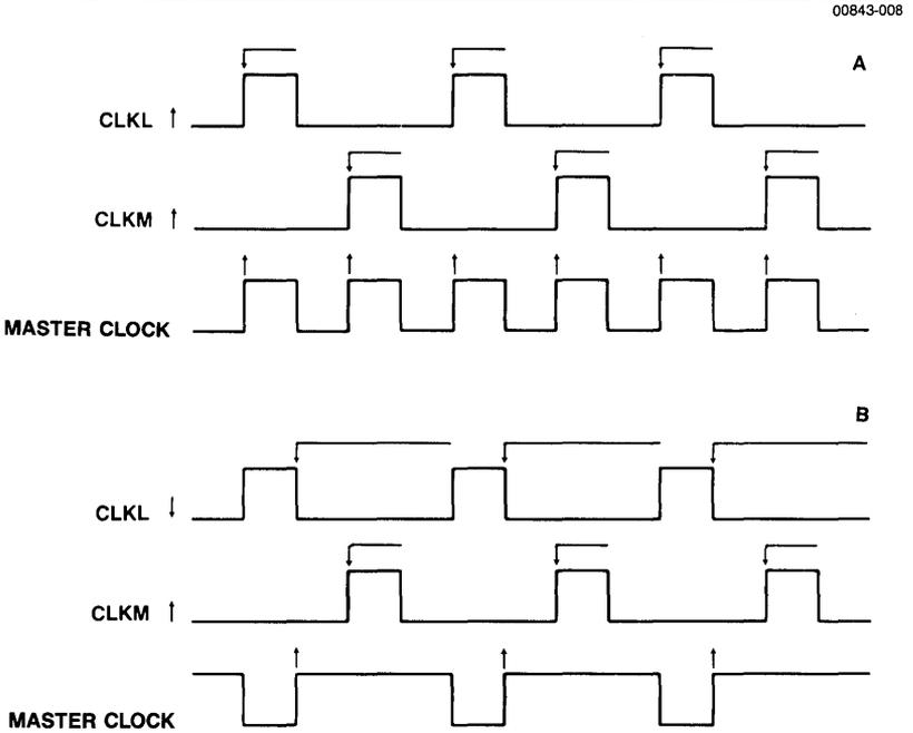
■ Figure 4-2. The effects of clock polarity.
