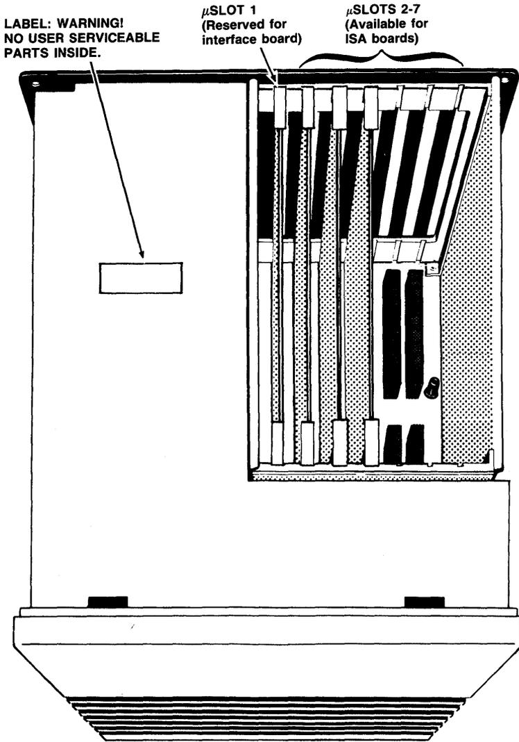
■ Figure 2-11. The mainframe's card cage.
