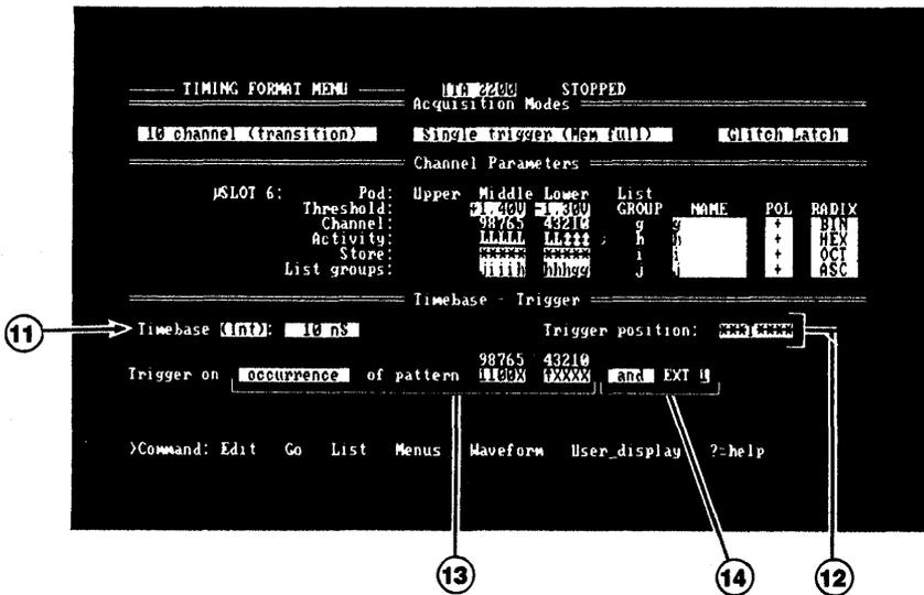
■ Figure 5-7. The Format Menu and its fields for controlling the timebase—trigger.
