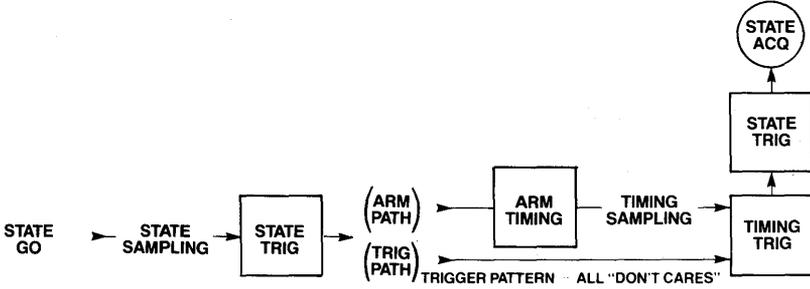
Figure 6-8. State Arms/Triggers Timing, Timing Triggers State.
