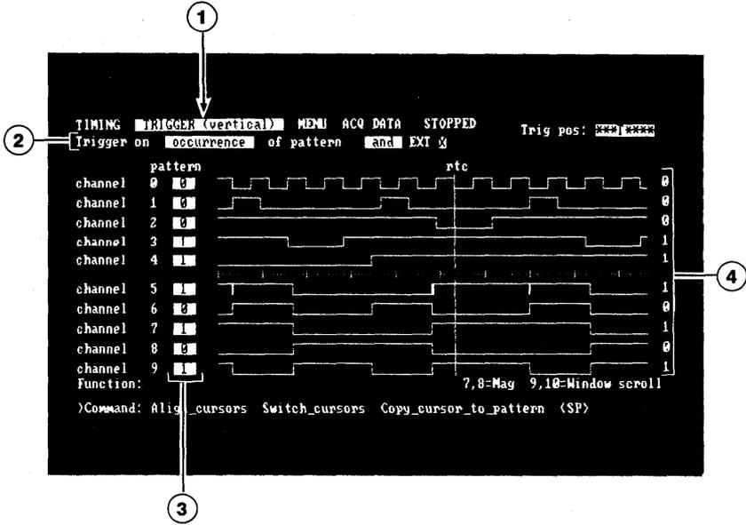
■ Figure 5-18. The Trigger\_find(vertical) Menu and its fields for defining a trigger pattern.
