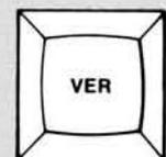
Press the VER mode key, then use steps 1, 2 and 3. The display will show a rapid scan of Copy addresses and Buffer data, Copy PROM data is displayed in the binary display next to the Copy socket on the Personality Module. If a mismatch occurs the M900B display will halt showing address of mismatch and data. Press ENTER to proceed with the verification, or select a new mode or RESET.
