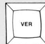
Press the VER mode key, then use steps 1, 2 and 3. The display will rapidly show Master addresses and data in sequence, then "F" (Finished) if all data compares. If the display halts, the data and address from the Master PROM are displayed. Use LIST to determine Buffer data, or press ENTER to proceed with the VER operation.
