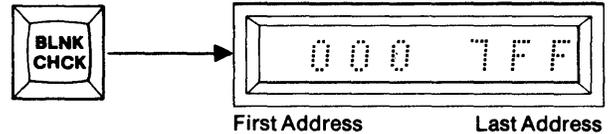
4. To Blank Check the entire contents of the Master PROM, starting with the first location, go to step 5. To Blank Check a limited field, continue. Use the hex keyboard to key in a new Start Address, MSD first. Repeat for the Ending Address.
