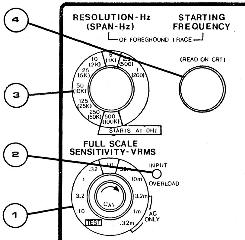
Fig. 2-1 The 3-Knob Cluster: Sensitivity, Resolution (Span) and Starting Frequency
