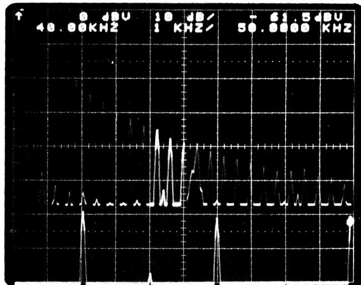
Fig. 2-2 BACKGROUND (dimmer intensity): 0 - 100 KHz with selected 10 KHz SPAN (brighter intensity)
