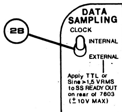
Fig. 2-10 The Data Sampling Control
