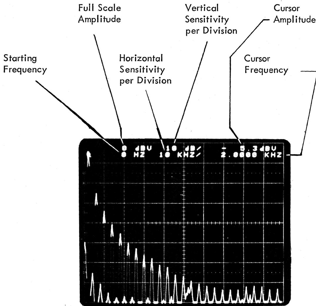
Fig. 4-1 Spectrum of the Test Signal
