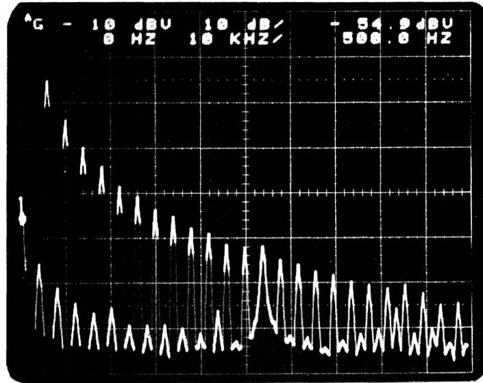
Fig. 4-8b Effect of 10 dB of Spectrum Gain; Spectrum Gain = 10 dB
