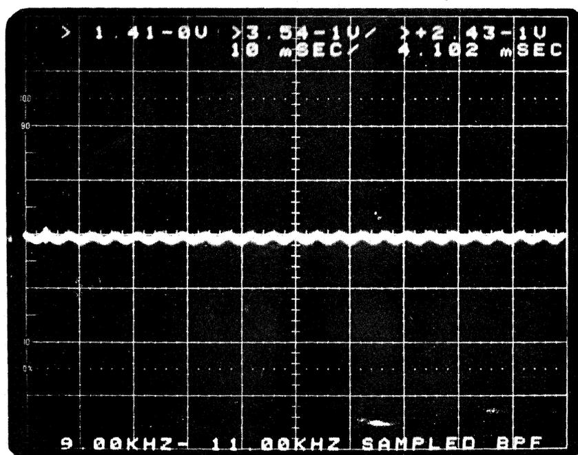
Fig. 4-7b Time Display of Test Signal, 9 - 11 KHz SPAN
