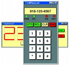
The Virtual Interface Panel (Viper) allows you to build custom user interfaces for your embedded applications using drag-and-drop virtual hardware components. Viper is ideal for rapid prototyping and experimentation. You can also use Viper to develop custom user interfaces for debugging and testing applications. A single Viper can communicate over the network with multiple Chameleon sessions allowing you to control multiple processors at different locations at the same time.
