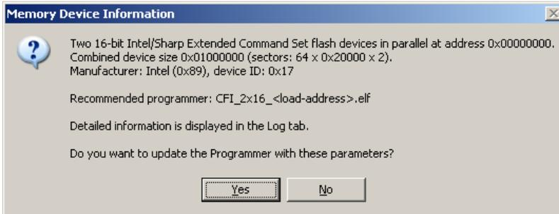
**FIGURE 3** Flash query using the Query Device button. The results can be used to configure the Programmer automatically.
